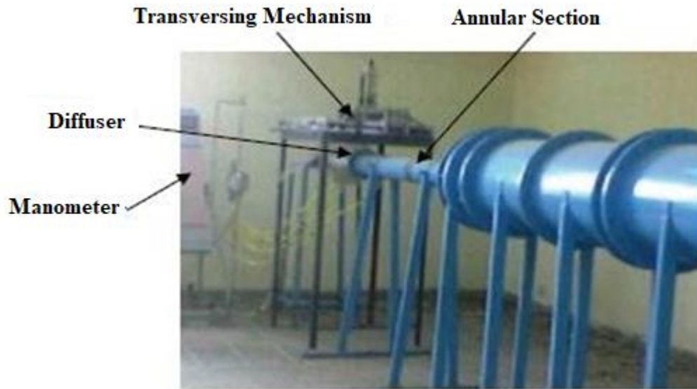
Figure 3.1: Actual experimental setup of the diffuser.
