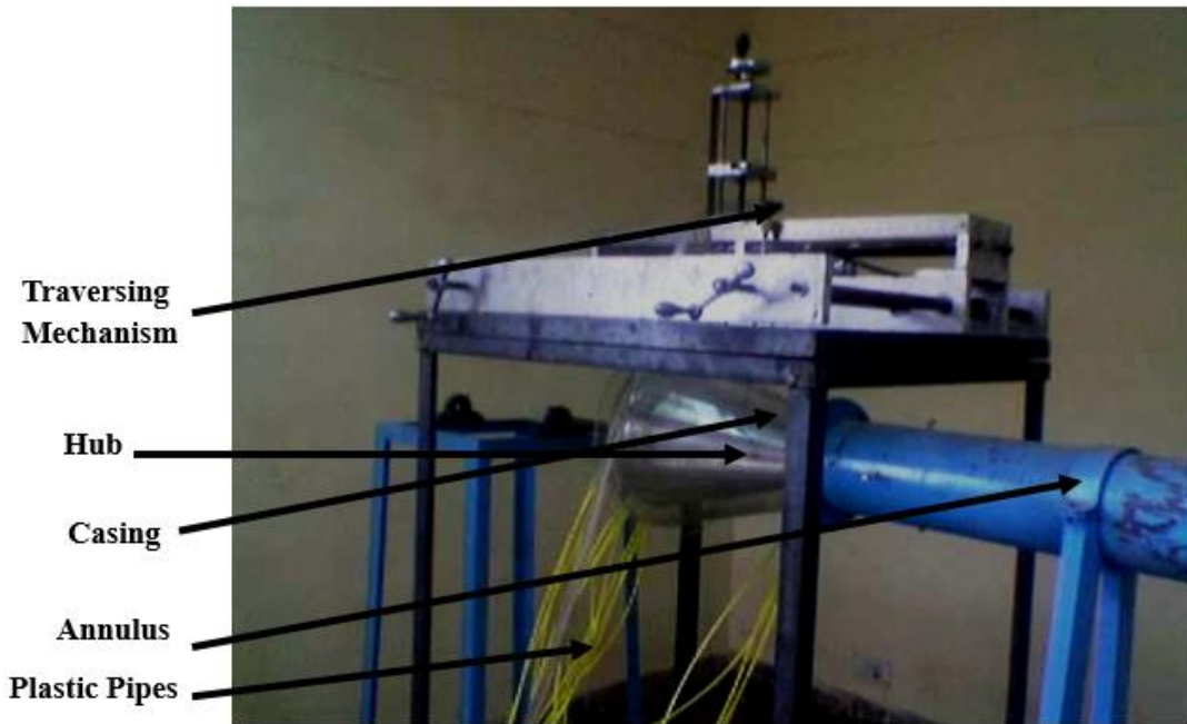
Figure 3.4: Traversing mechanism for the experimental setup.
