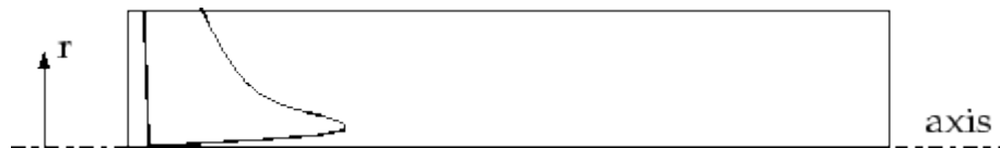
Figure 1.7: Free vortex flow of \omega in the radial direction (Source: Fluent user's guide (2014)).
