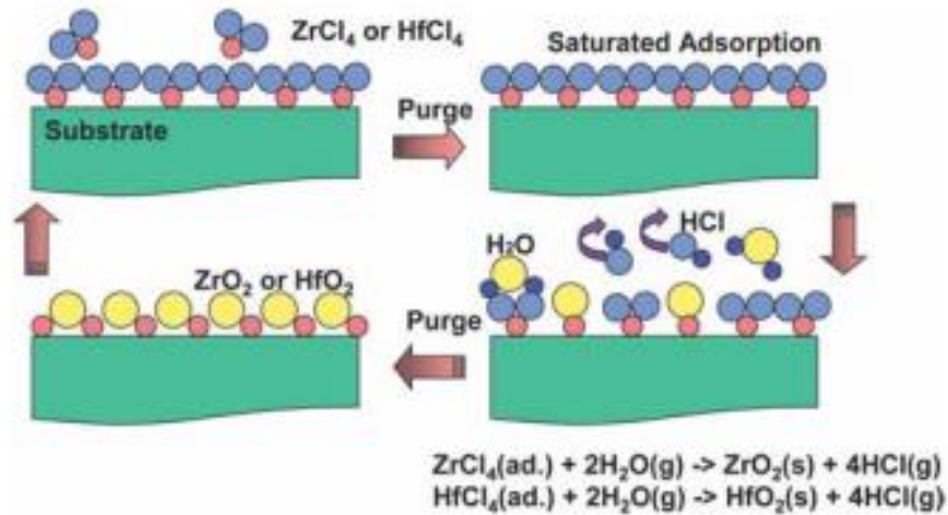
Fig 12: Schematic of the cyclic process of Atomic Layer Deposition.
