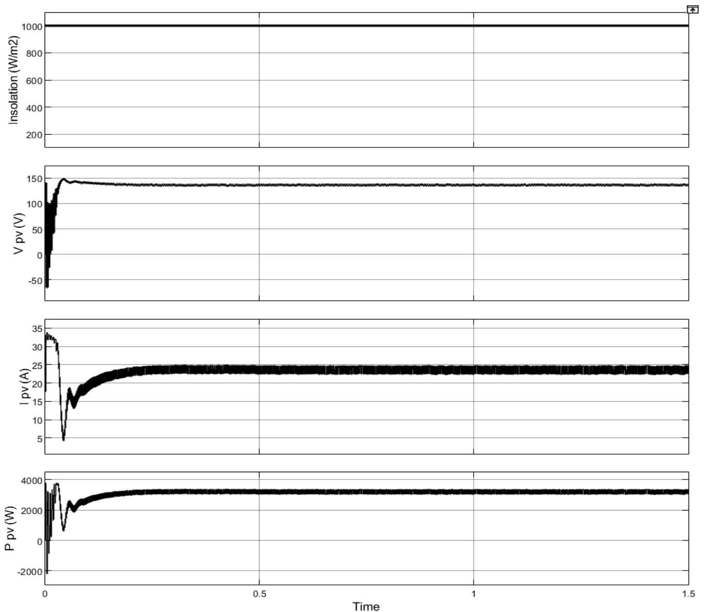
Fig. 14. SPV array peak insolation output at 1000\text{W/m}^2 .
