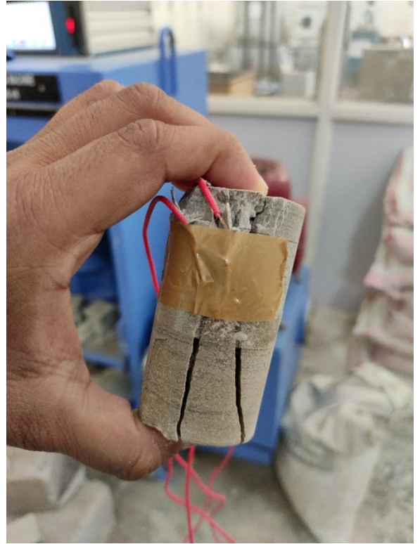
Fig:39 progression of crack across the plane
