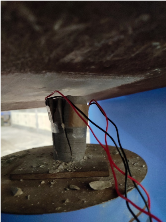
Fig:38 failure of sample with recording stress and strain
