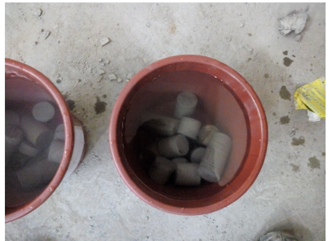
Fig:17 Samples placed in saline environment
