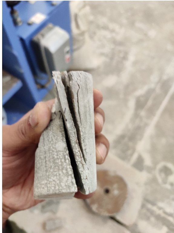
Fig:41 bedding plane at an angle of 75°
