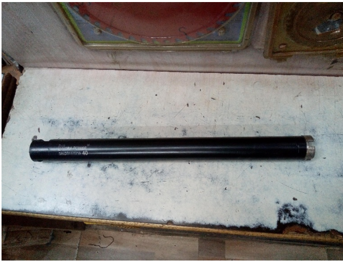
Fig:11 Drill bit ( \varnothing = 44\text{mm} )
