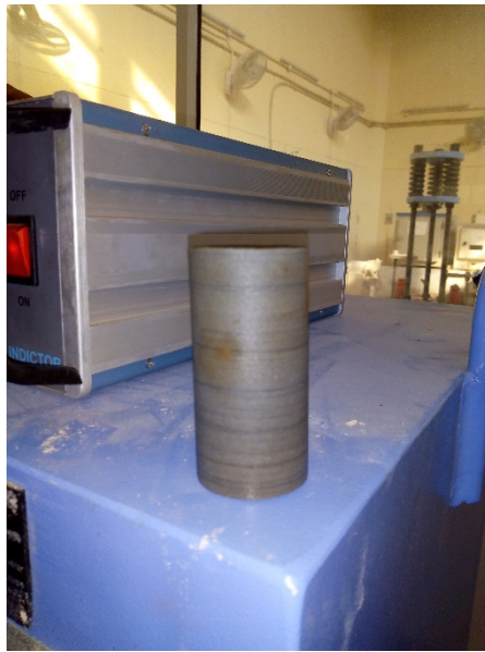
Fig:27 0-degree bedding plane
