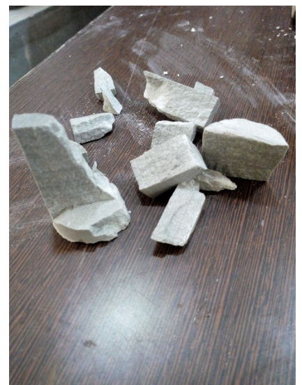
Fig:21 failure in UCS
