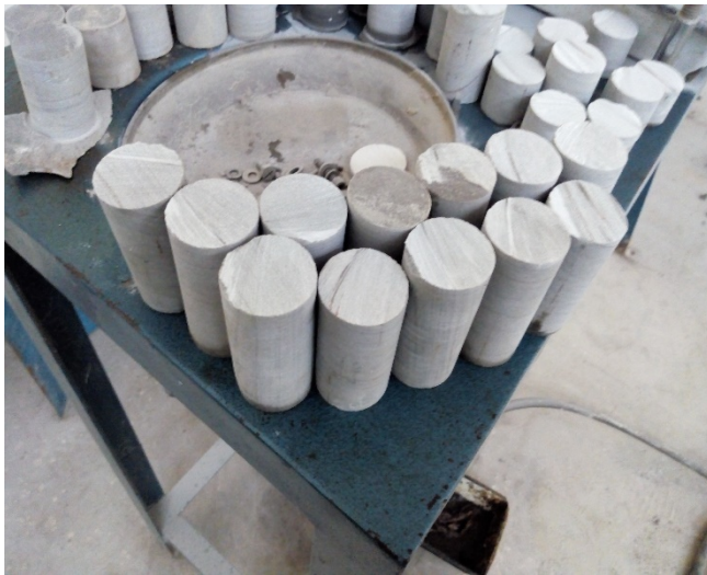
Fig:14 Core samples of standard dimension
