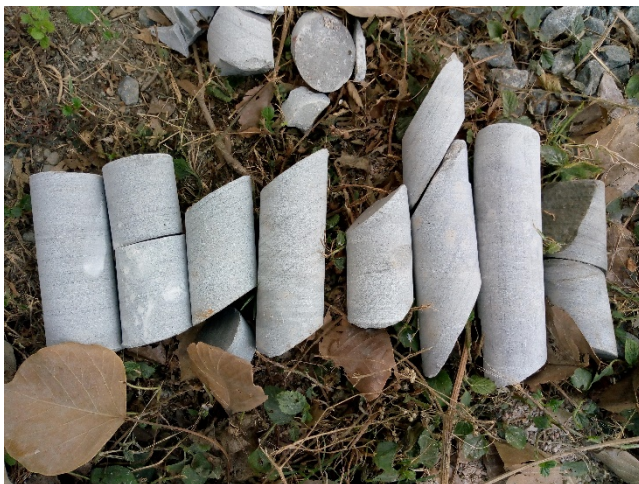
Fig:13 Samples with bedding planes
