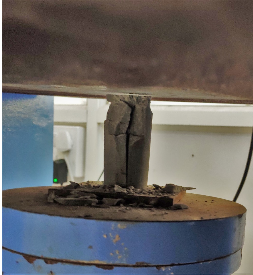
Fig:42 failure along the bedding plane for 10% NaCl
