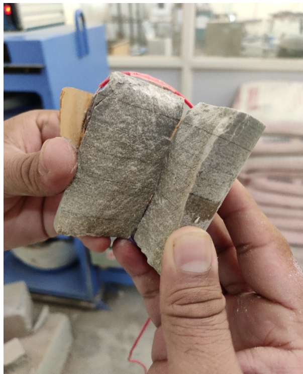
Fig:40 failure plane across the bedding plane of the sedimentary rock
