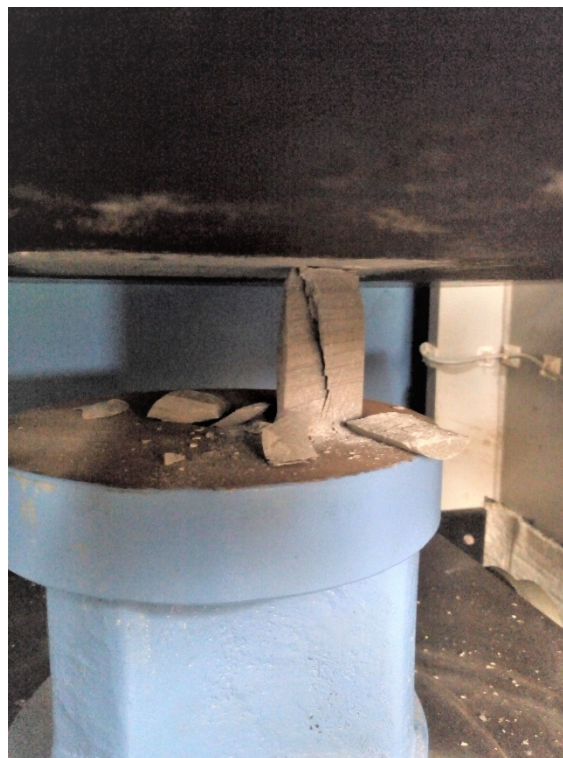
Fig:28 progression of crack across the plane
