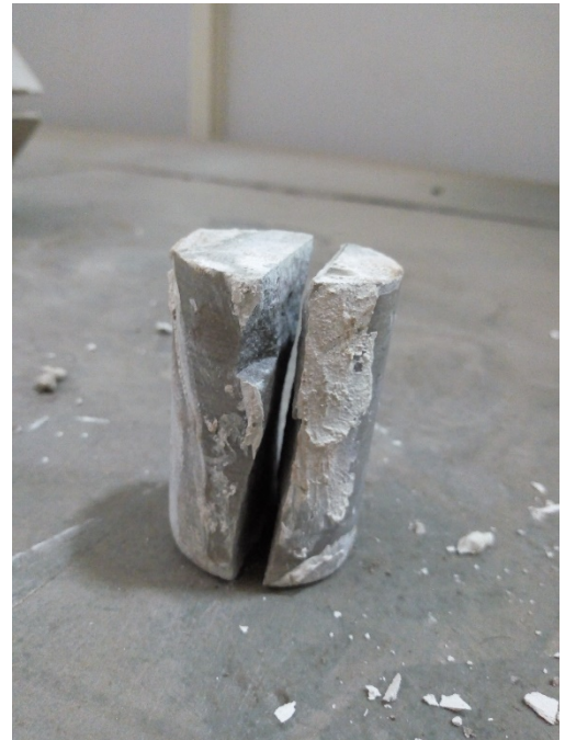
Fig:23 oblique shear failure
