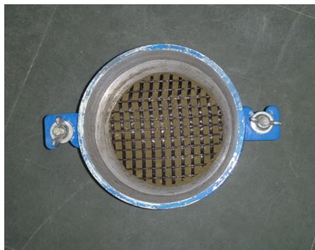
Figure 3.3 Orientation of reinforcement layer placed at predetermined depth in CBR mould
