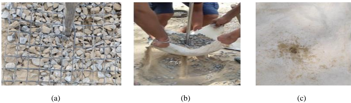
Figure 5.12 Condition of geosynthetics after DCP test: (a) Deformed shape of geogrid; (b) easy to separate aggregates due to the presence of geotextile for the removal of DCP rod after test; (c) deformed shape of geotextile.
