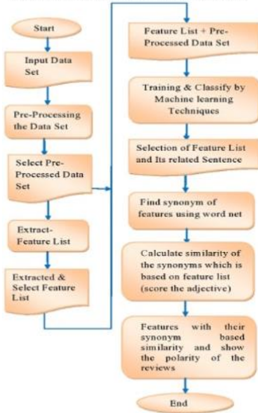
Fig. 2. Flow Diagram of the proposed methodology
