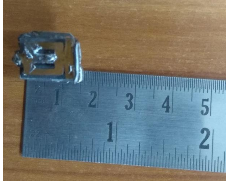
Figure 5.7: Fabricated absorber-loaded slotted PIFA antenna.
