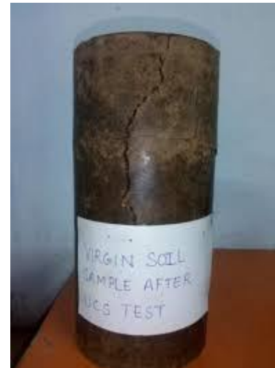
Figure 3.9 Plain Soil sample after UCS
