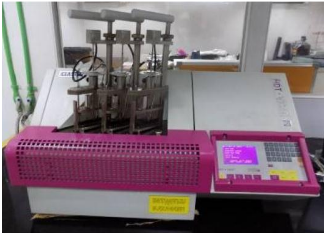
Figure 3.13: Heat Deflection Temperature (HDT) and Vicat Softening Temperature (VSP) make Ceast model HV3
