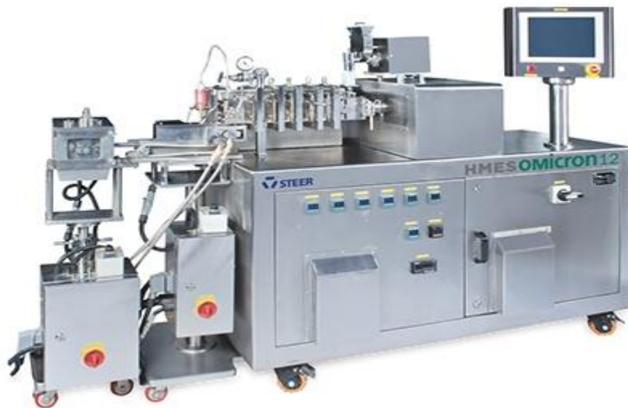
Figure 3.5: Lab Scale Co-rotated Twin Screw Extruder Steer India make.
