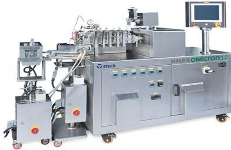
Figure 4.3: The co-rotating Twin Screw Extruder used for melt reactive blending.
