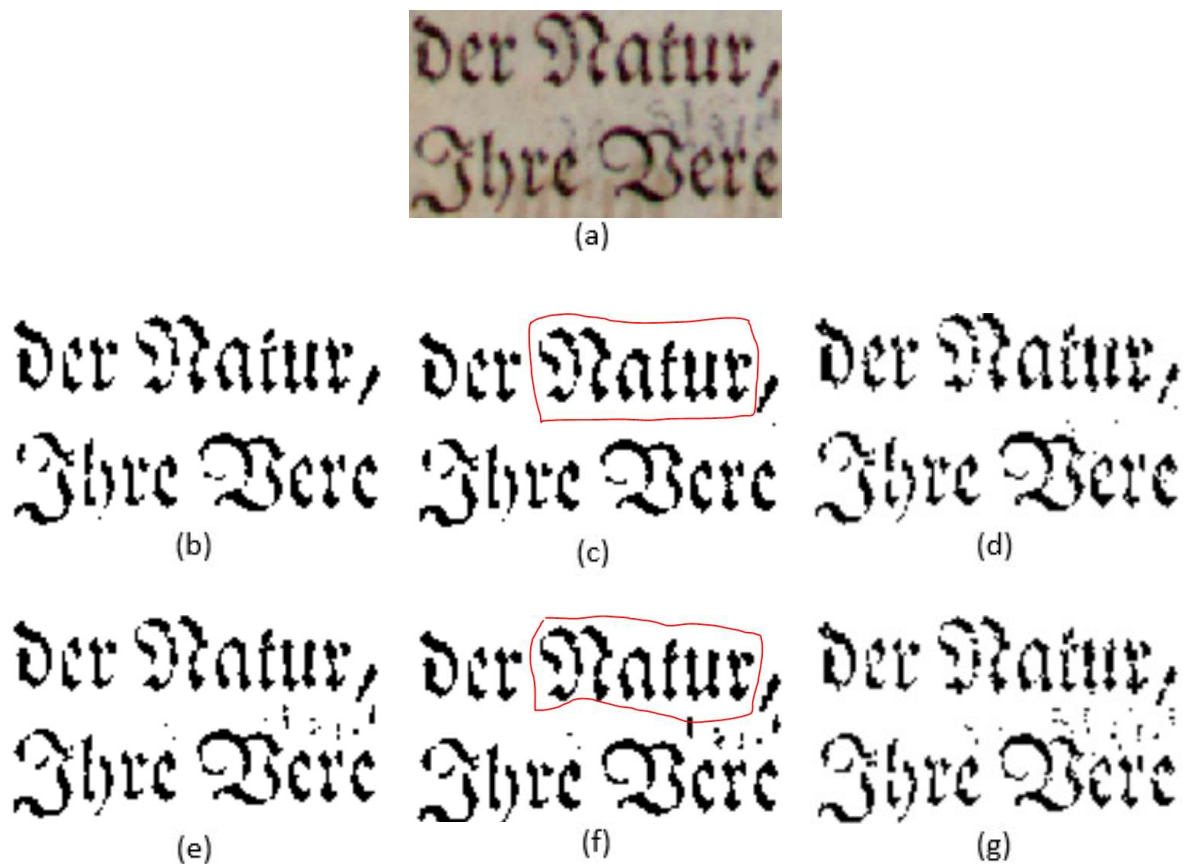
Fig. 4.7 a) Input image (5 th image from DIBCO-2009 Printed) b) Sauvola , c) Spd -Sauvola, d) Cprgb2gray -Sauvola, e) Nick, f) Spd-Nick , g) Cprgb2gray -Nick
