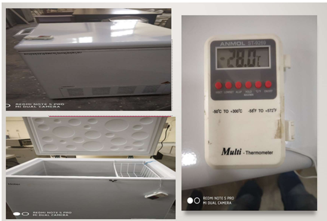
Fig. 3.29 Picture of deep-freezer with temperature meter
