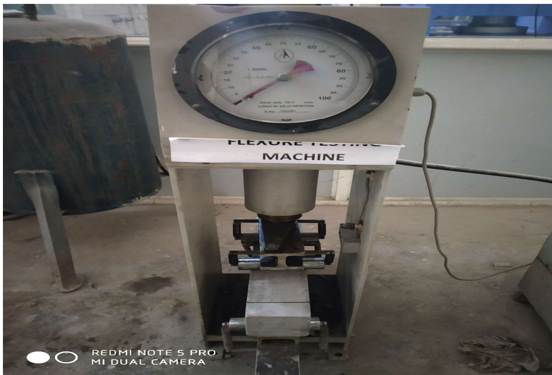
Fig. 3.21 Picture of the flexural strength test setup during testing
