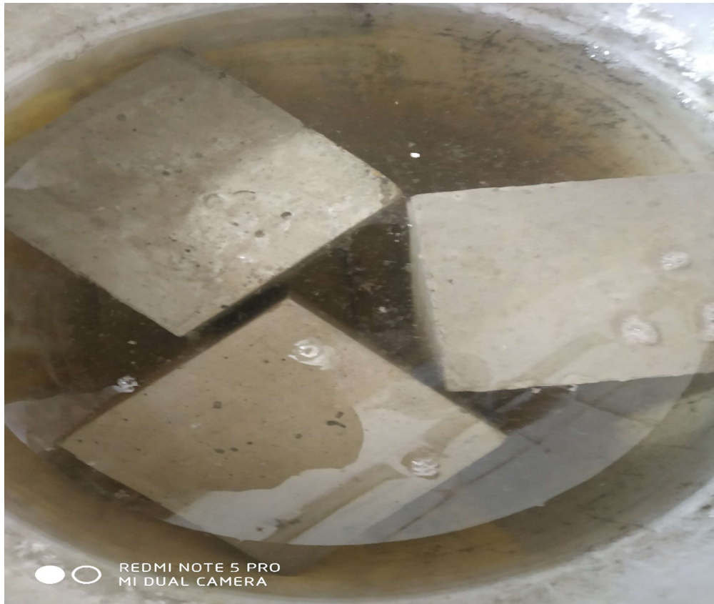
Fig. 3.27 Picture of seawater solution with the cube specimens
