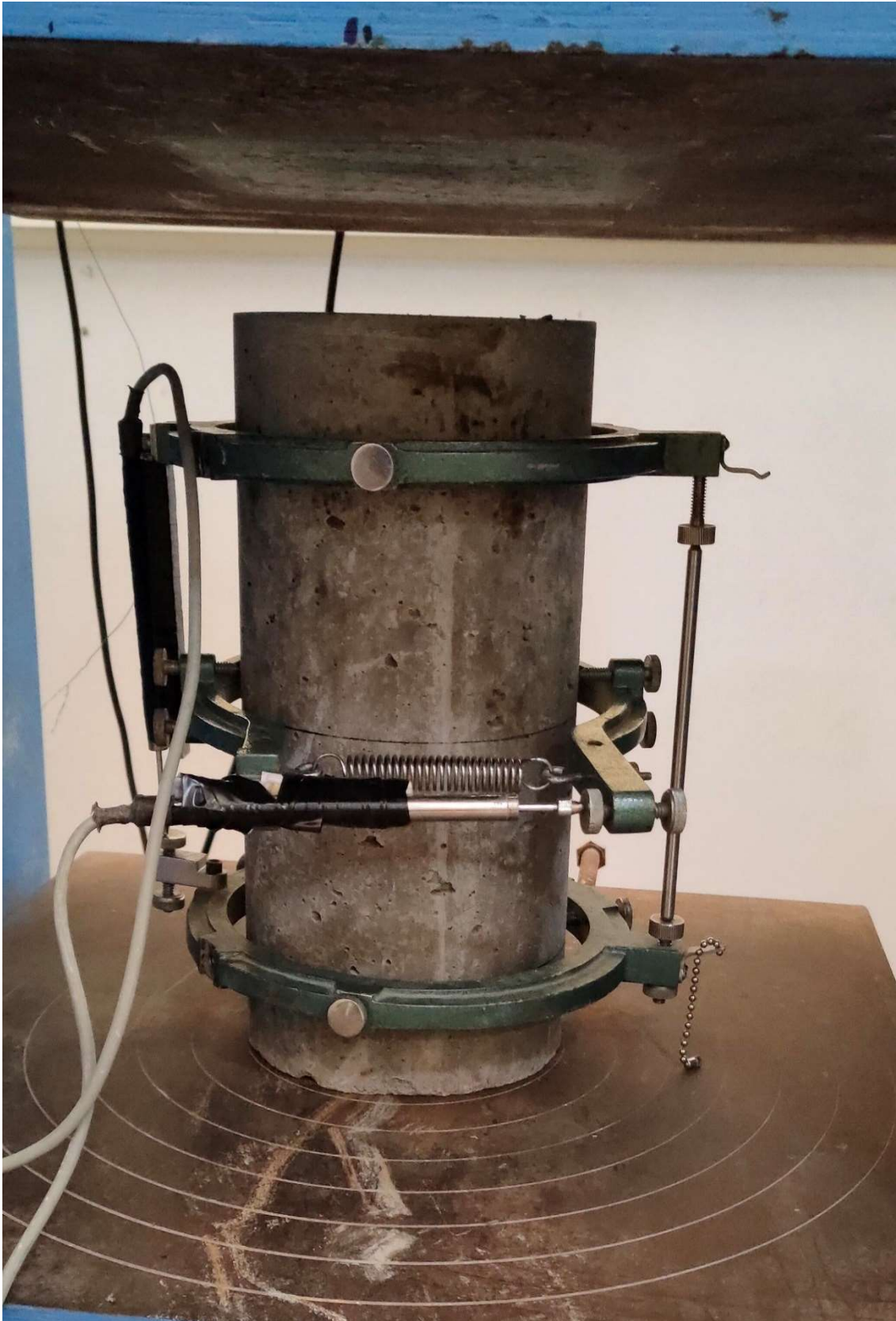
Fig. 3.22 Elastic modulus and Poisson's ratio test setup
