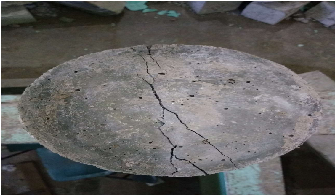
Fig. 3.20 Picture of splitting tensile failure of the specimen
