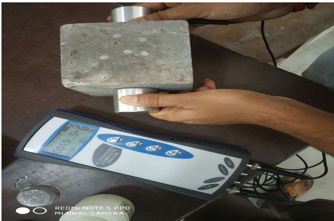
Fig. 3.24 Picture during UPVT conduction
