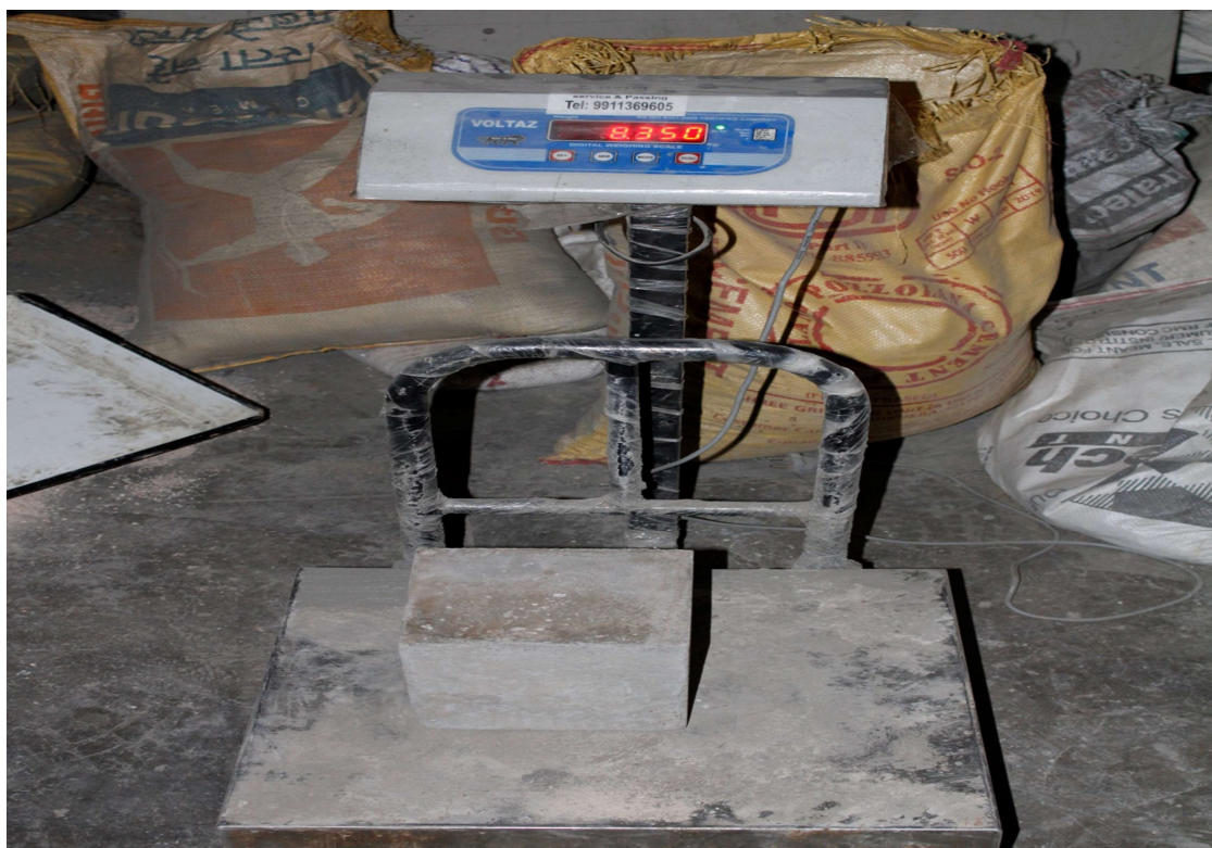
Fig. 3.18 Digital weight machine for finding density by weight of the cube
