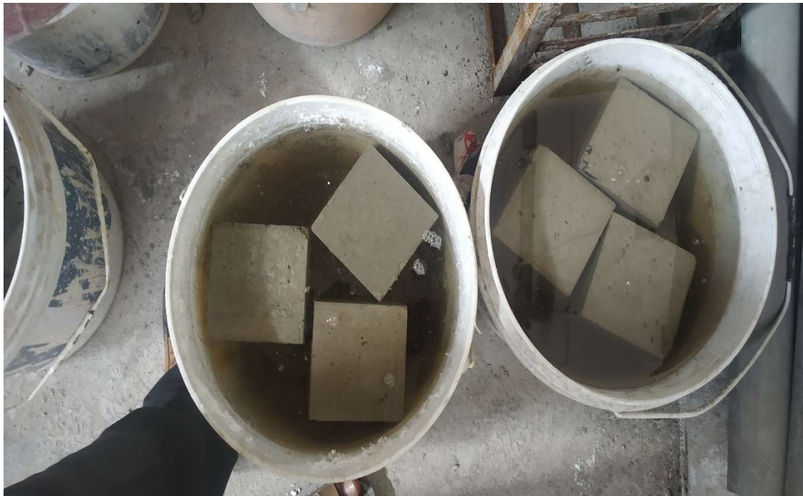
Fig. 3.28 Picture of sulphate solutions with the cube specimens
