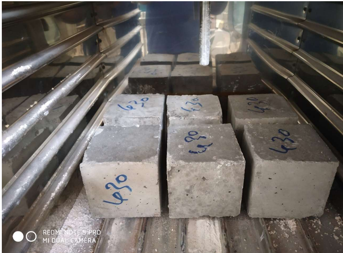
Fig. 3.17 Specimens during oven-curing
