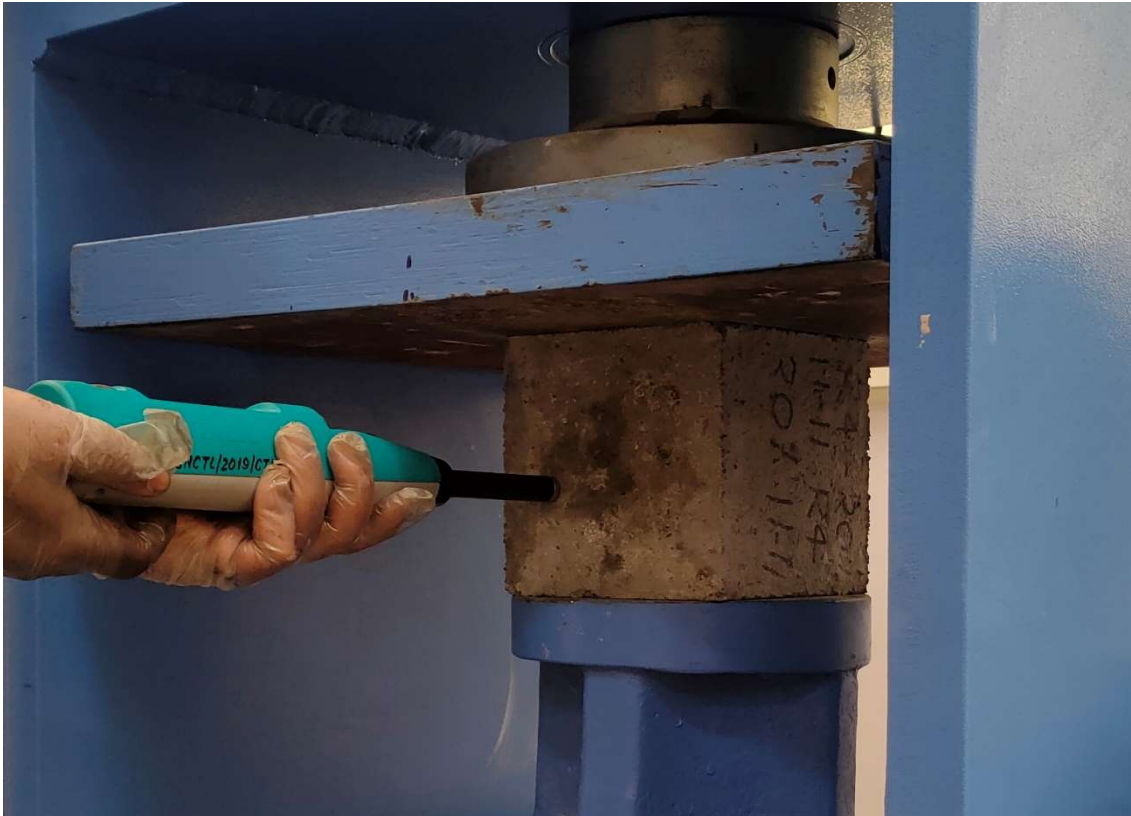
Fig. 3.23 Picture during rebound hammer strength test
