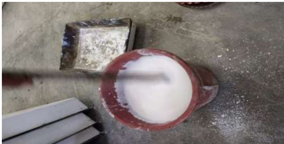
Figure 4.2: Nano particles being mixed with water and super plasticizer
