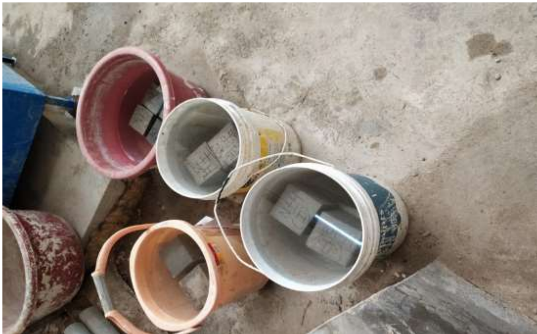
Figure 4.8: Some specimen being cured in combined sodium sulphate and sodium chloride
