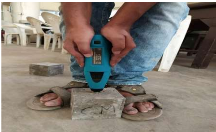
Figure 4.11: Rebound hammer Test being performed
