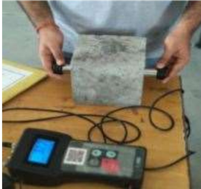
Figure 4.12: UPV test being performed
