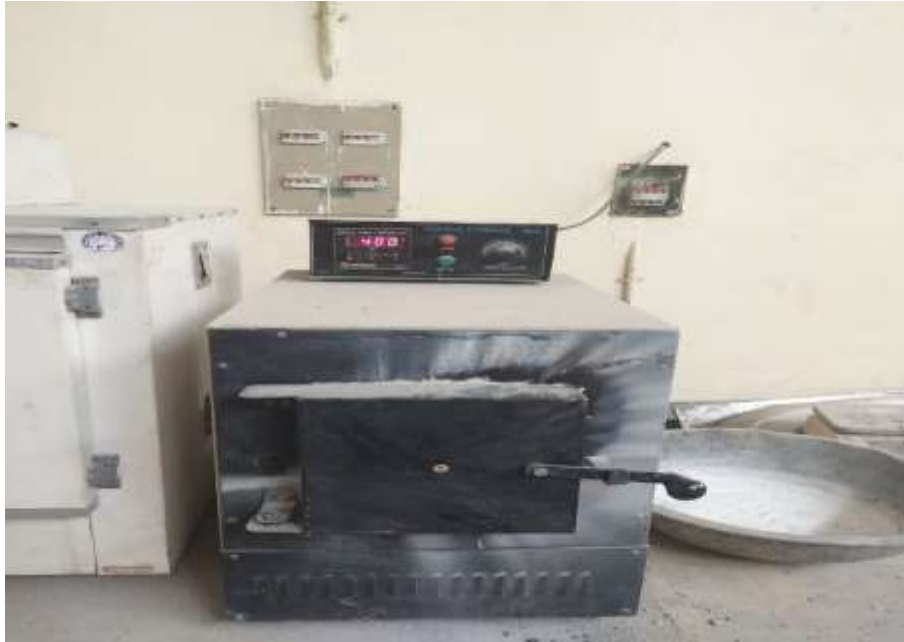
Figure 4.16: Specimen being heated at 400°C in muffle furnace
