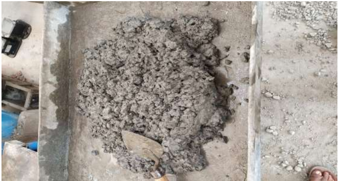
Figure 4.4: Concrete after mixing
