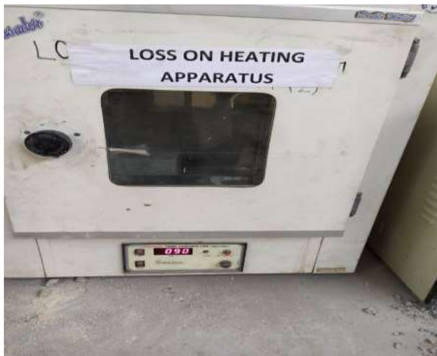
Figure 4.15: Specimen being heated at 90°C in oven
