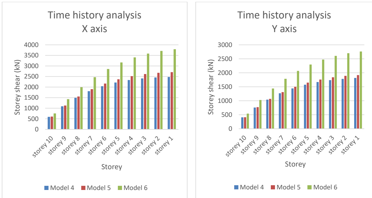
Figure 4. 12 Storey shear graph using time history analysis in X and Y direction without shear wall.
