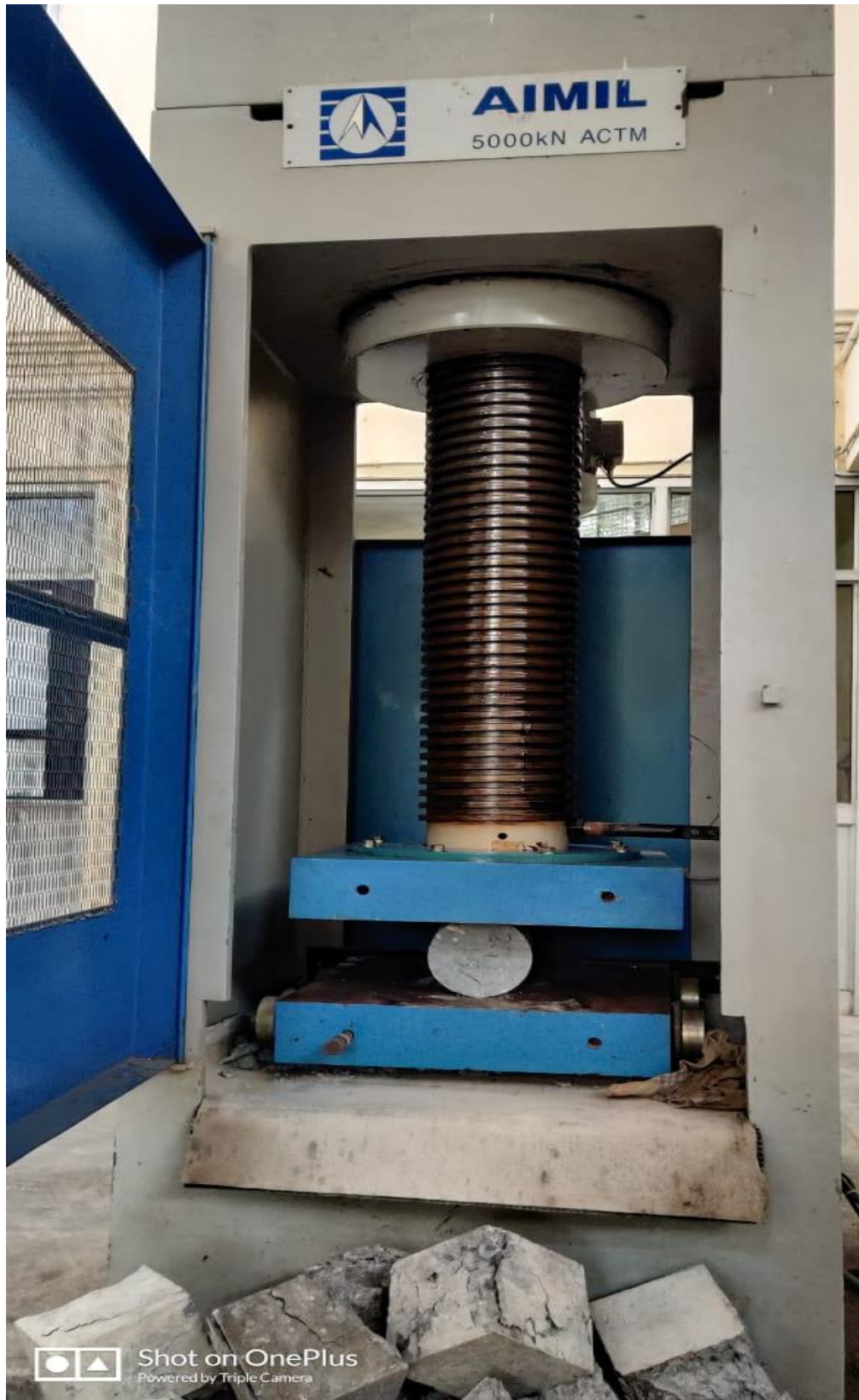
Figure 5.5: Performing Split cylinder test on compressive testing machine.
