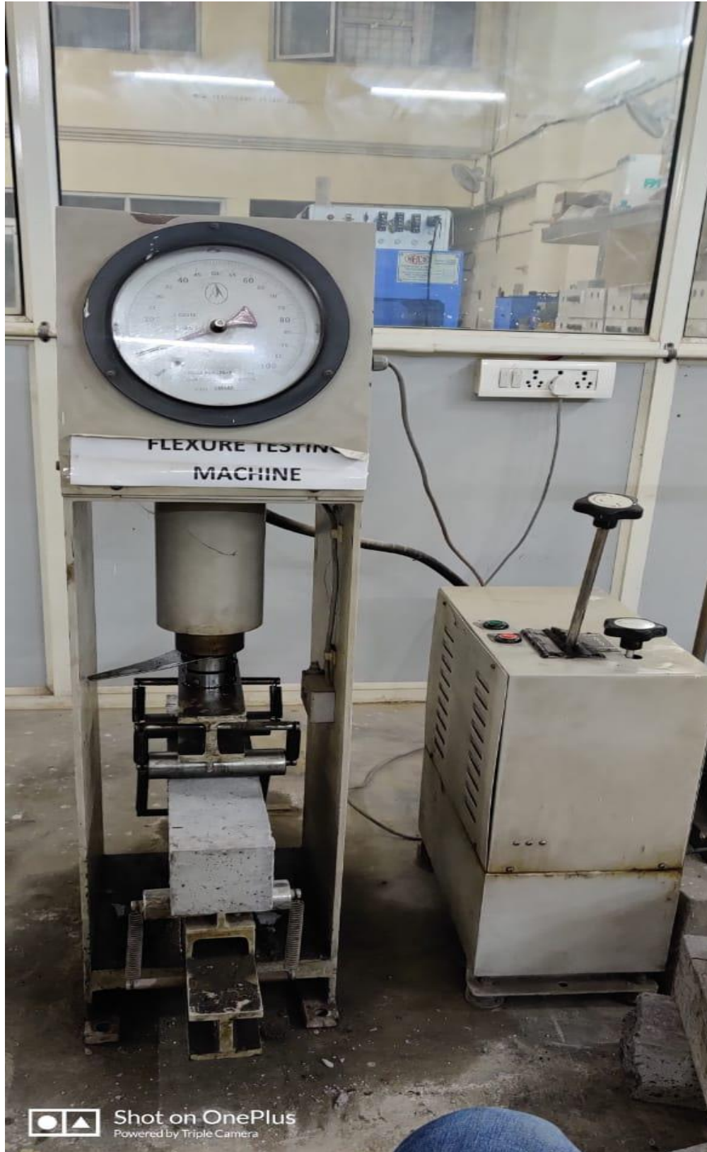
Figure 5.4: Flexural testing machine performing test on beams.
