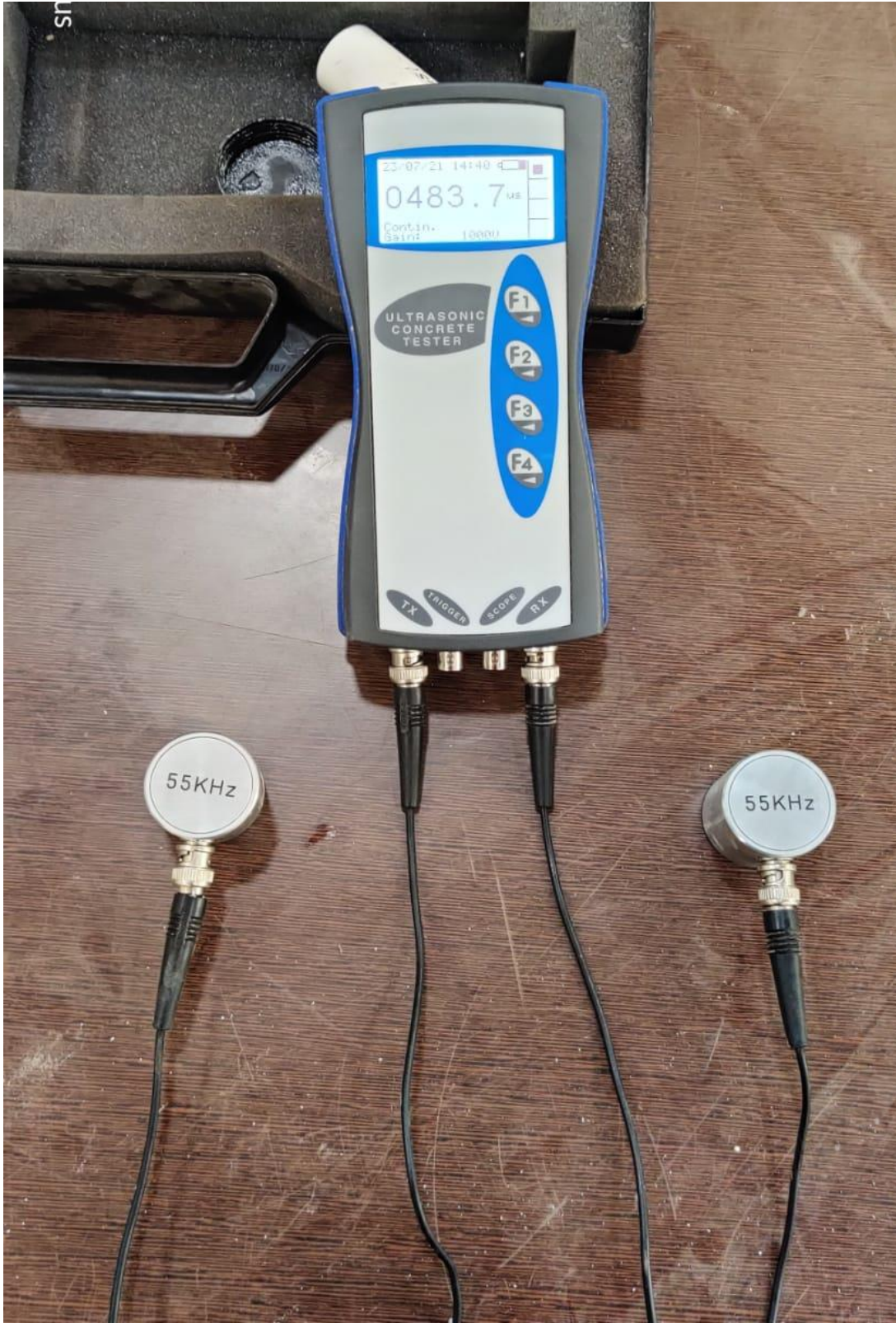
Figure 5.8: Ultrasonic Pulse velocity test setup.
