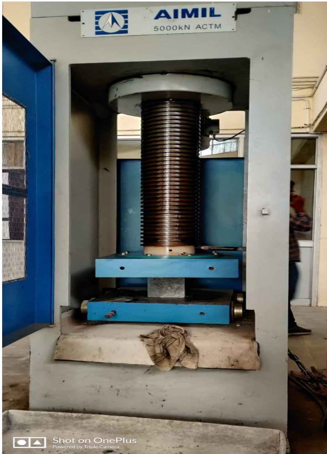
Figure 5.3: Compressive testing machine of 5000KN capacity.
