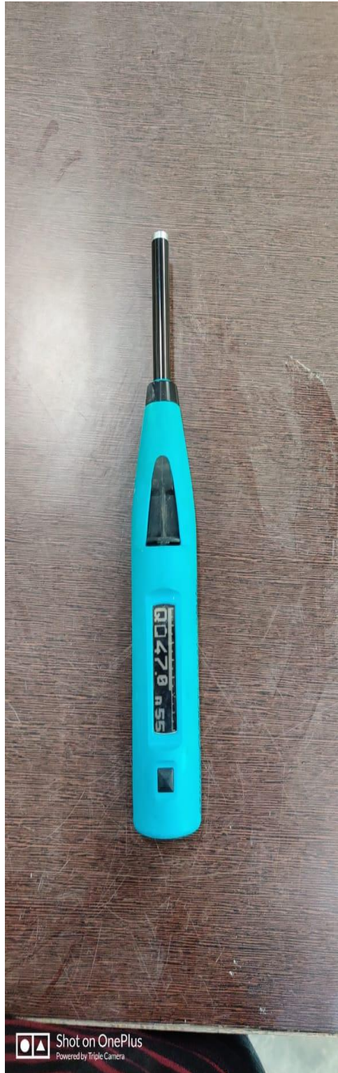
Figure 5.6: Digital Rebound hammer. Figure 5.7: Performing Rebound hammer test.
