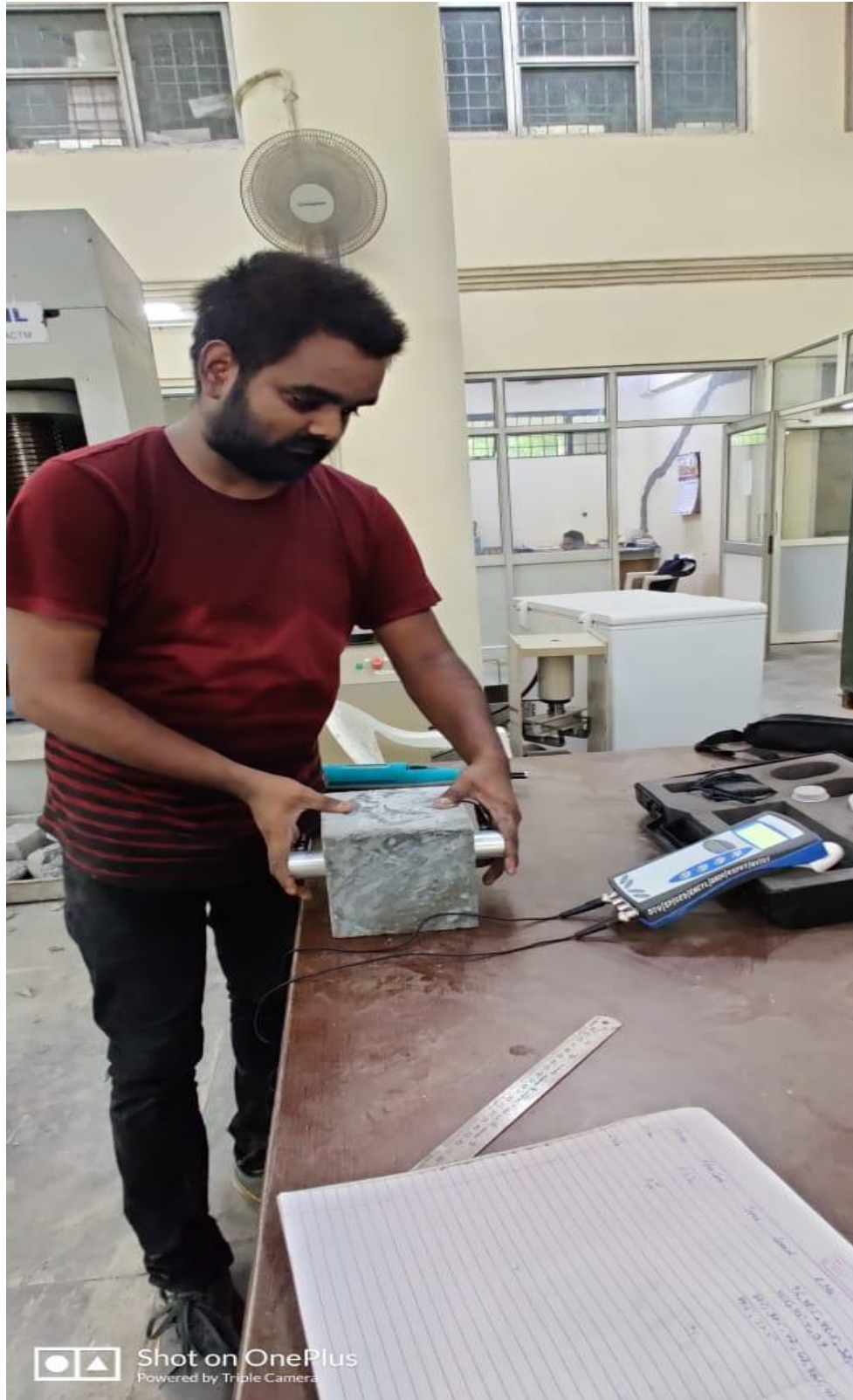
Figure 5.9: Performing Ultrasonic pulse velocity test on cube specimen.
