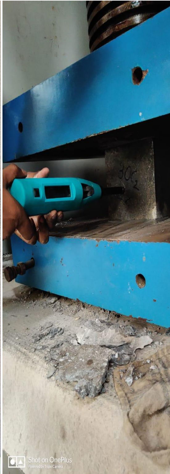
Figure 5.6: Digital Rebound hammer. Figure 5.7: Performing Rebound hammer test.
