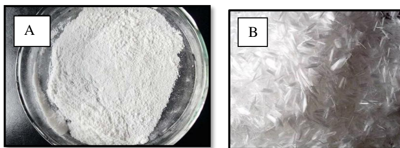
Figure 6: (A) HDPE (B) Nylon 6,6 fibers
