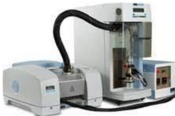
Figure 3.6: Perkin Elmer thermo gravimetric analyzer TGA 4000
