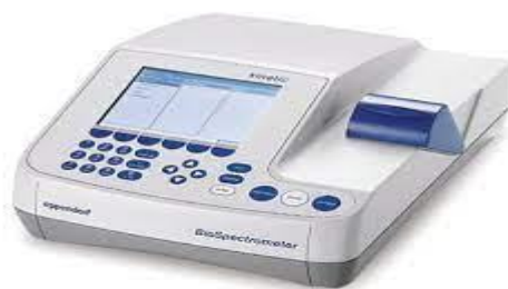
Figure 3.3: Eppendorf UV-Vis Spectrophotometer for analysis of Optical Density
