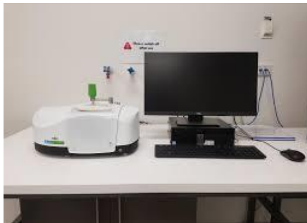
Figure 3.5: Perkin Elmer Spectrum 2 FTIR system
