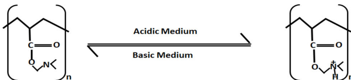
Figure 2.1 Hydrogel Containing Acidic Hanging Groups
