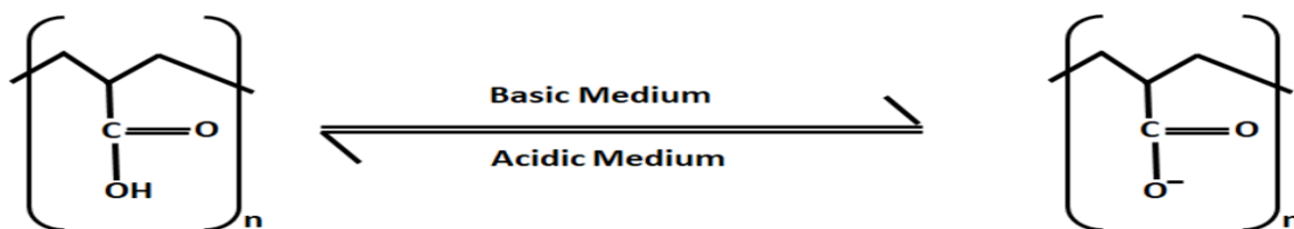
Figure 2.1 Hydrogel Containing Acidic Hanging Groups
