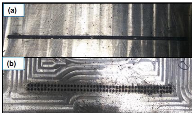
Figure 4.22 (a, b)-The groove and holes for filling of the nanoparticles reinforcement
