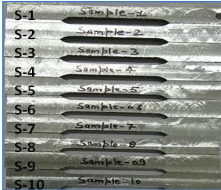
Figure 4.24- Tensile test samples cut from the composite region
