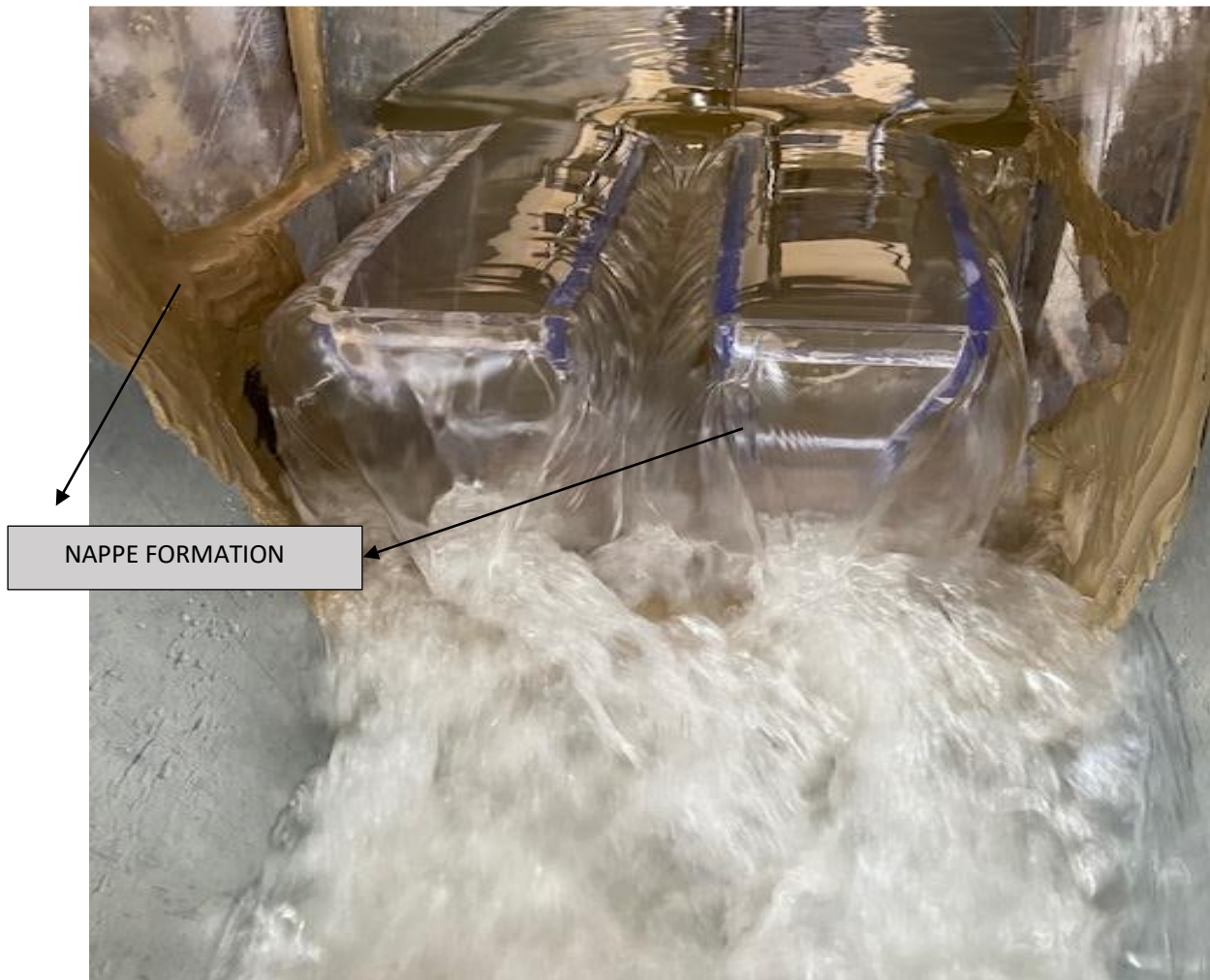
Fig-3.9 (a) and (b) showing flow and nappe formation over Type-A P K Weir
