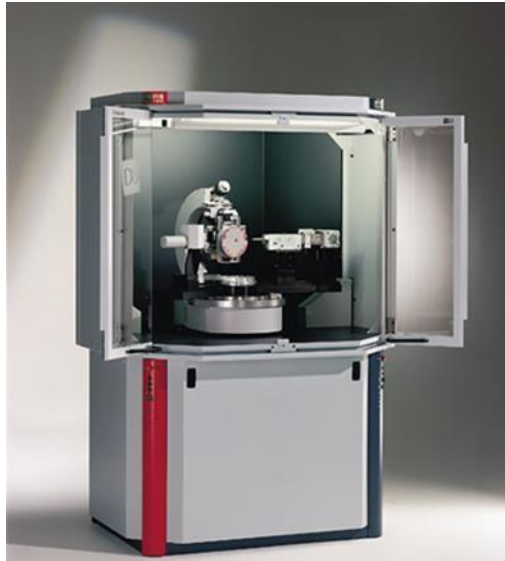
Fig. 4.2 X-ray Diffractometer [Model: Bruker's D8 Discover] in DTU.
