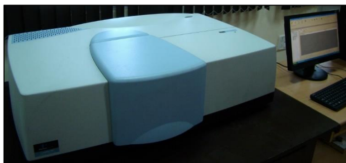
Fig. 4.3 UV-Vis-NIR Spectrophotometer (Model: Perkin Elmer 750 LAMBDA) [86].
