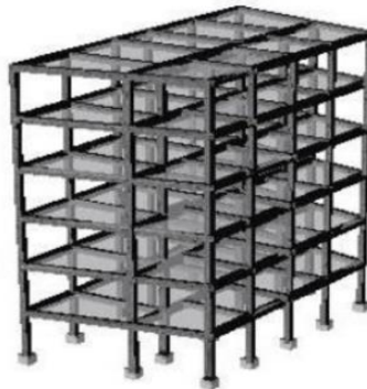
Fig 1.3 Bare Frame of a Building
