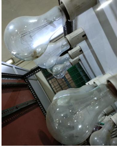
Plate 3.9: Electric Bulb used for Loading purpose
