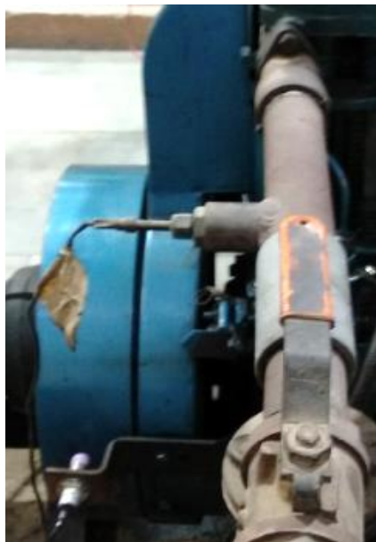
Plate 3.11: Thermocouple attached to the exhaust manifold
