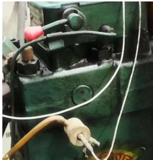
Plate 3.12: Pressure transducer attached to the engine
