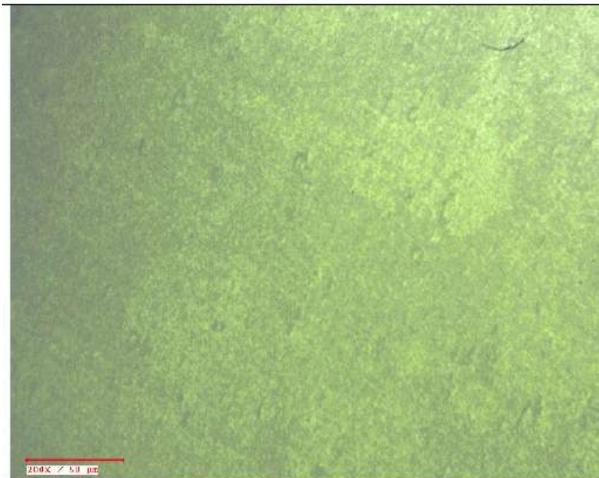
Figure 5.79: Optical microscope image at 600 rpm, 65 mm/min, R1, RS at 200X
