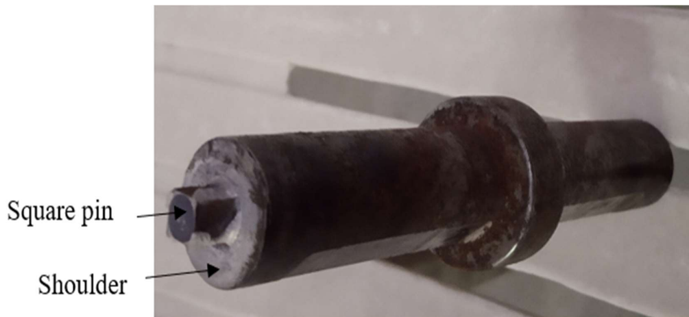
Figure 4.2: FSW tool after welding
