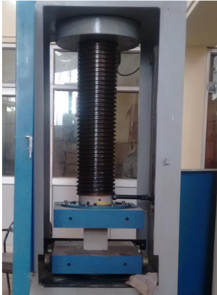
Fig. 3.12 (e) Concrete Cube in CTM for testing
