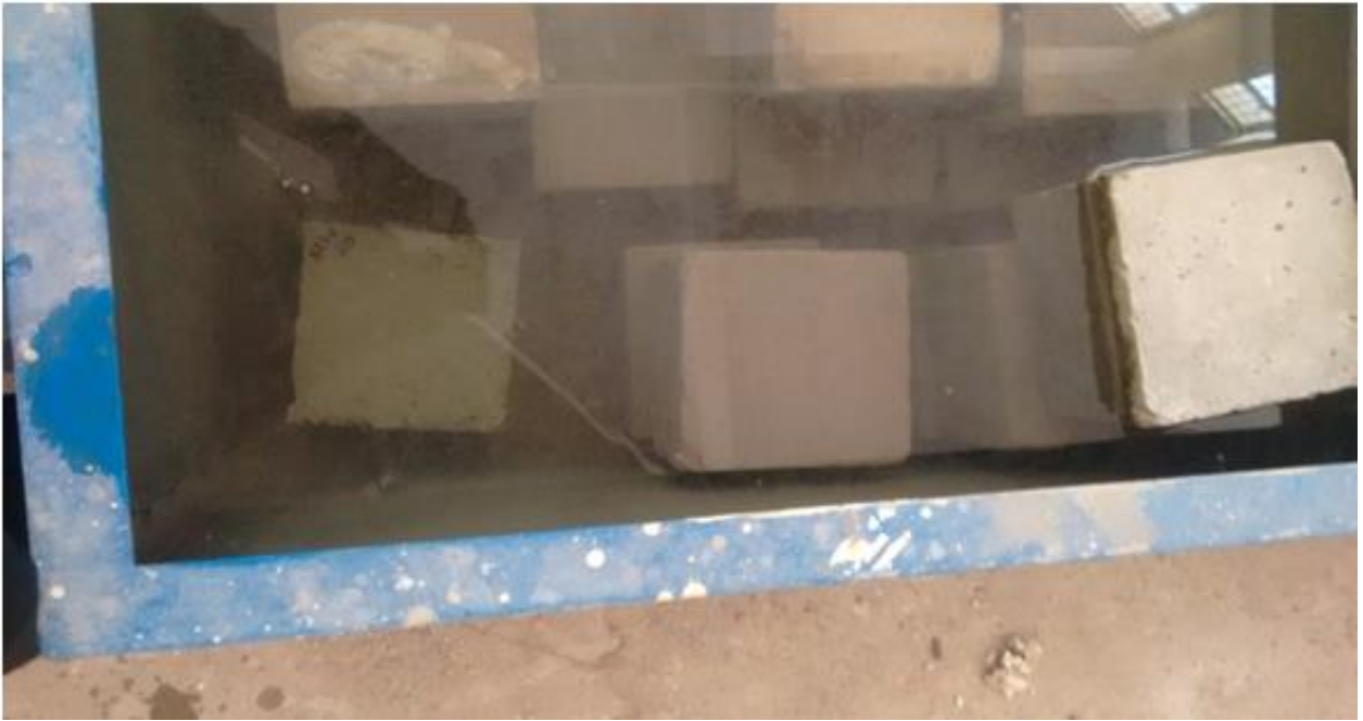
Fig. 3.12 (c) Concrete cube placed inside curing tank for 28 days
