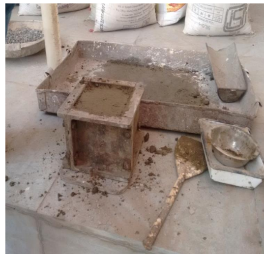
Fig. 3.12 (b) Placing of concrete in mould of size 150mm X 150mm X 150mm
