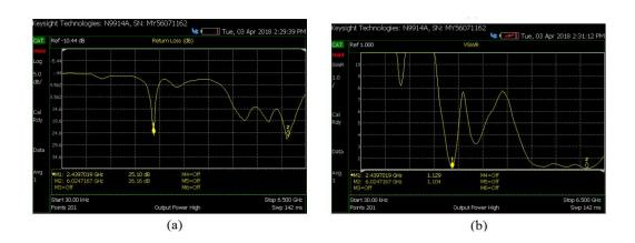
Figure 3.10: Measurement of (a) Return loss (b) VSWR on Keysight N9914A vector network analyzer.
