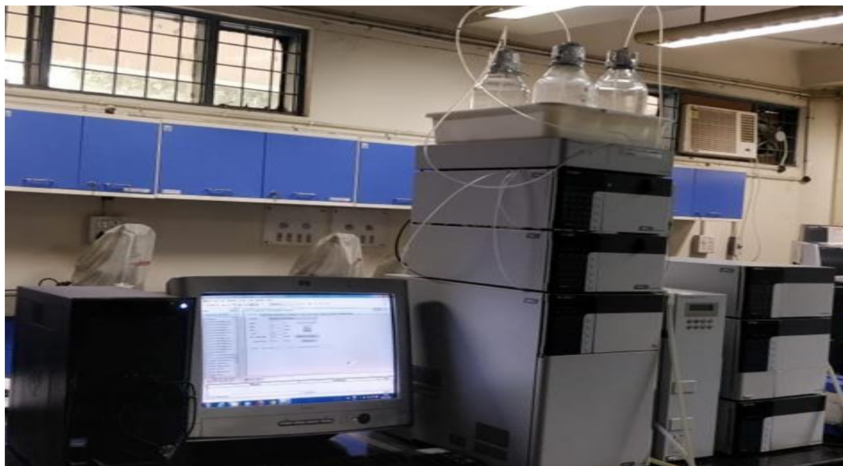
Figure 3.5. HPLC system (Shimadzu make) used for analysis of intermediates and concentration of pharmaceutical drugs
