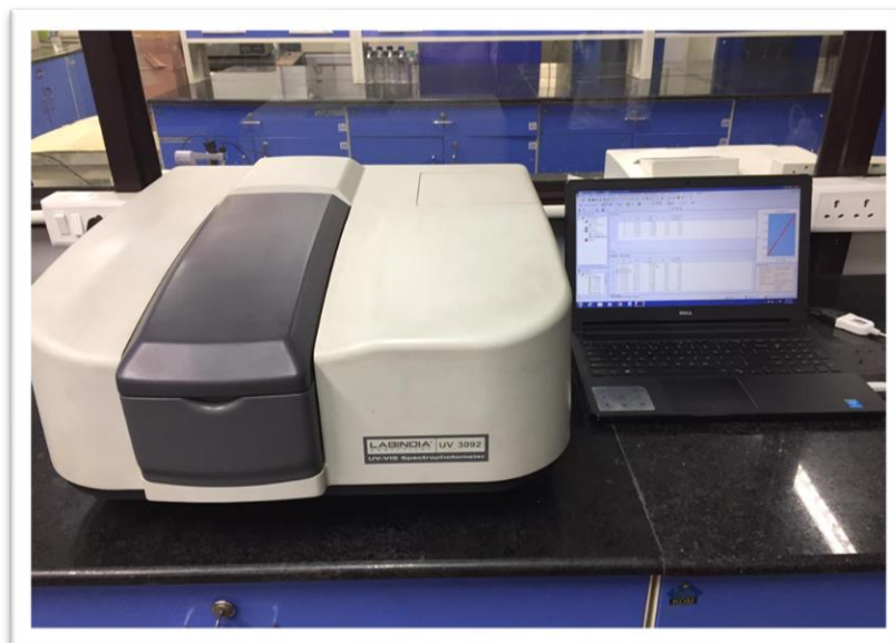
Figure 3.4. Double beam UV-Vis Spectrophotometer (Lab India make) used for determining the concentration of drugs in the present study
