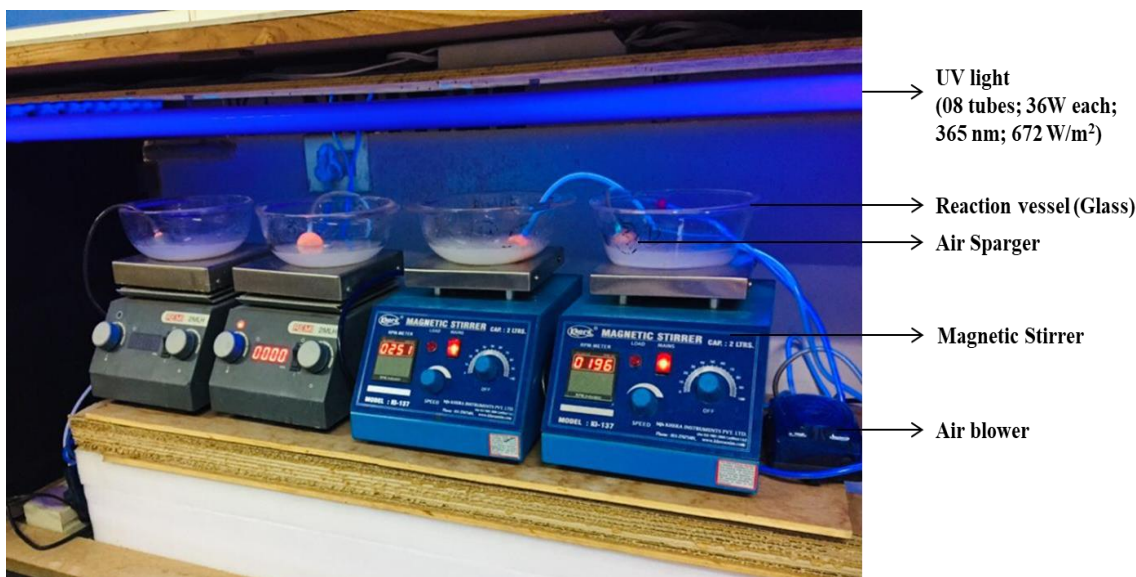
Figure 3.6. Experimental setup for photocatalytic degradation of AMX and ATL
