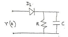
Determine the upper limit of RC to ensure that the capacitor voltage follows the envelope.
