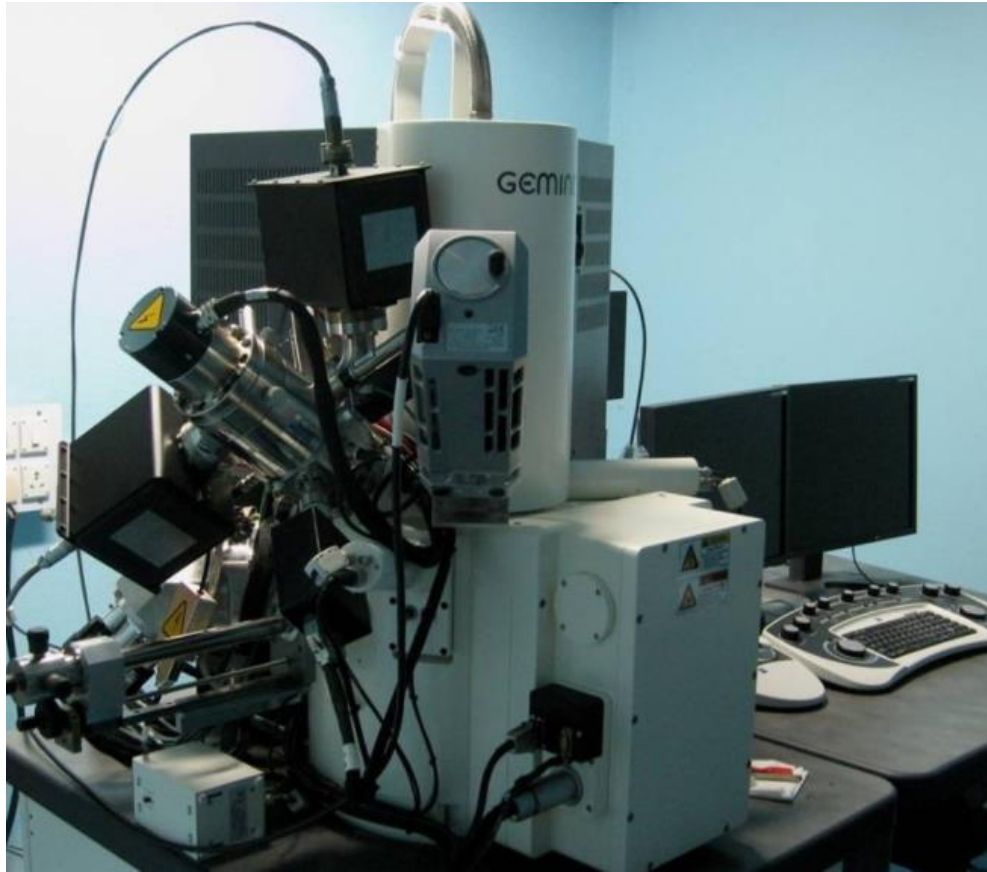
Figure 2.5 Photograph of FE-SEM, Gemini electron-optics
