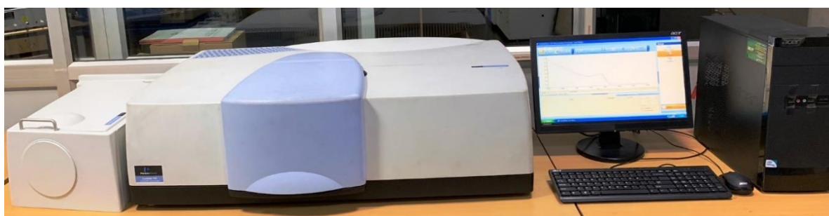
Figure 2.7 UV–vis spectrometer of PerkinElmer, Model- lambda 750.
