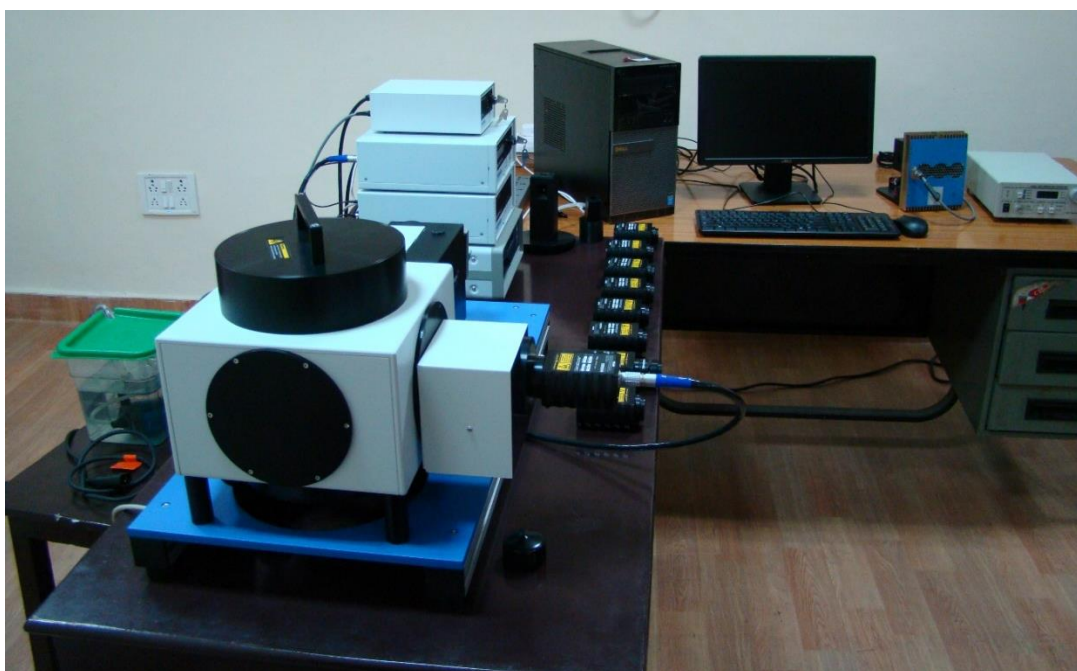
Figure 2.9 Photograph of TCSPC (DeltaFlex-01-DD) measurement unit.
