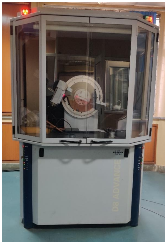
Figure 2.2 X-ray diffractometer (Bruker 8D advance)
