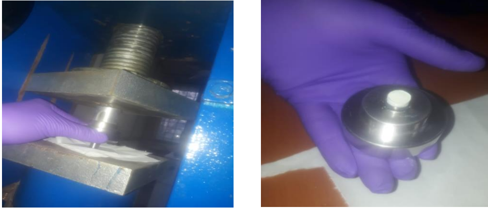
Fig. 2.2 Pellet formation by Hydraulic Press Machine using die set.
