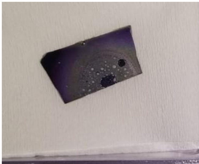
Fig 3: CVD grown MoSe 2 thin film on Si/SiO 2 substrate
