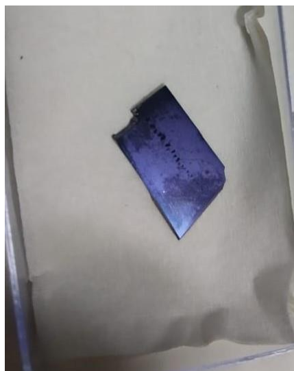
Fig 3: CVD grown MoSe 2 thin film on Si/SiO 2 substrate
