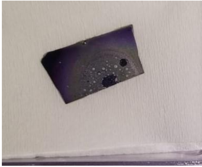
Fig 2.11: CVD grown MoSe 2 thin film on Si/SiO 2 substrate
