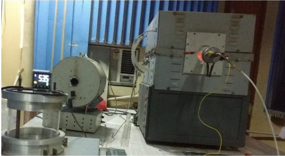
Fig 2.8: Thermal split furnace used for sample growth
