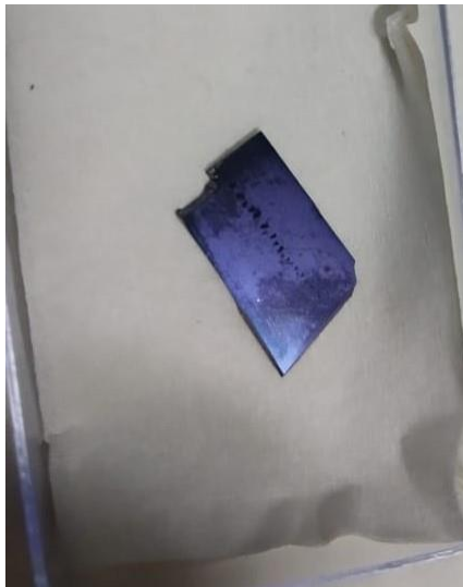
Fig 2.11: CVD grown MoSe 2 thin film on Si/SiO 2 substrate
