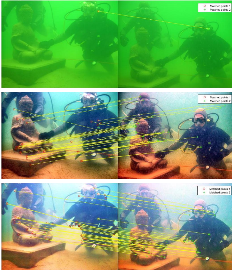
Figure 4.20: First row contains Original pair of images with only 2 SURF features are matching, second row contains enhanced pair of images using Ancuti et al. technique with 37 SURF features are matching and third row contains enhanced pair of images using FCCC with 48 SURF features are matching.
