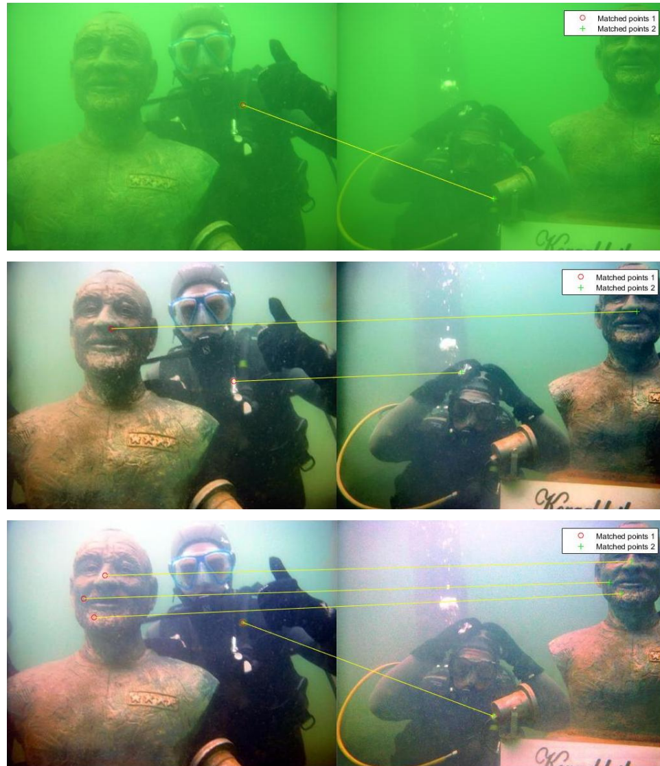
Figure 4.21: First row contains Original pair of images with only one SURF feature, second row contains enhanced pair of images using Ancuti et al. technique with 2 SURF features and third row contains enhanced pair of images using FCCC with 4 SURF features matching.
