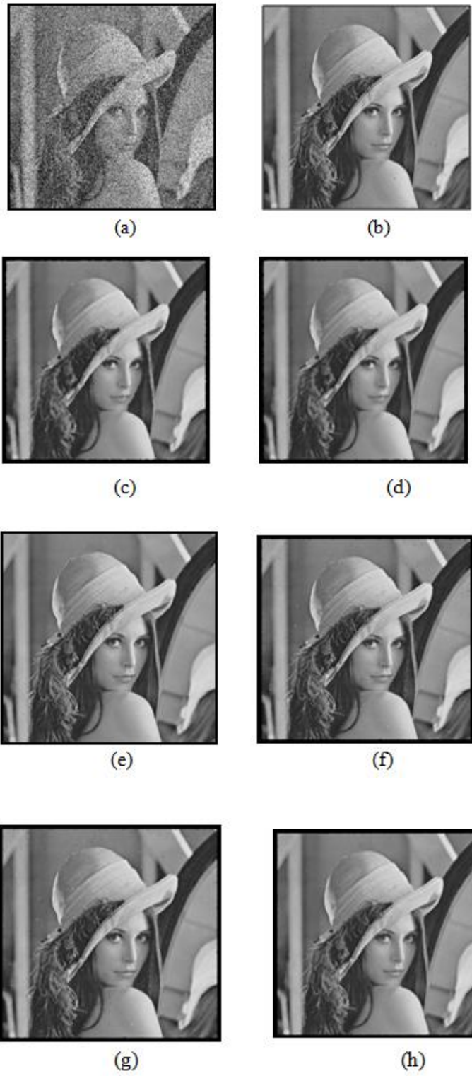
Figure 3.4 : Results for image “lena” using various methods (a) 30% Noisy image (b) ASWM (c) HEIND (d) EEP (e) MDBU (f) CEB (g) NAFSM (h) Proposed algorithm
