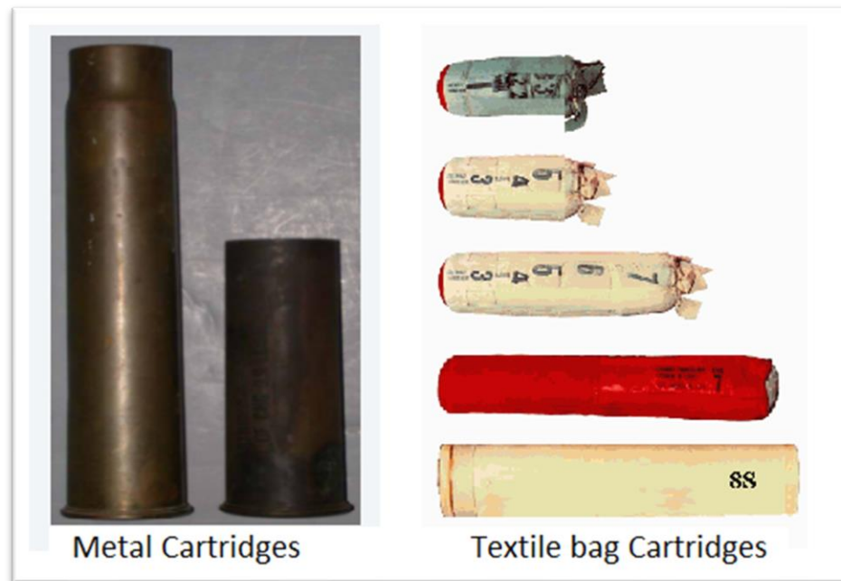
Fig. 1.3.1 Conventional Cartridges of Large Caliber Guns
