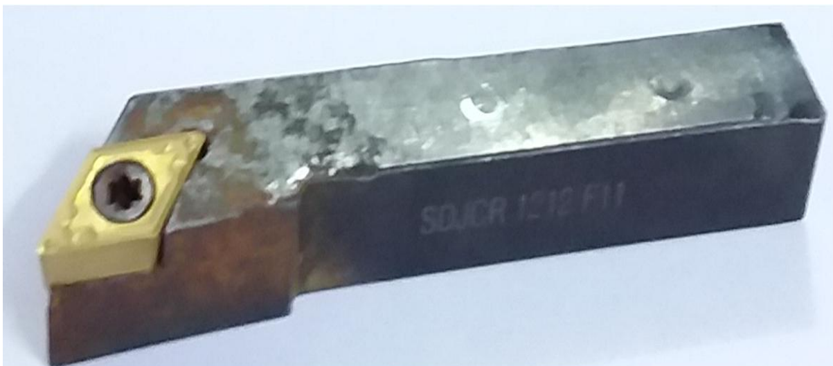
Figure 3.6 Single point cutting insert and tool holder
