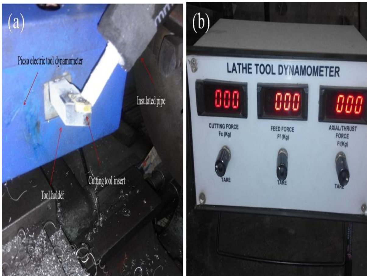
Figure 3.8 (a) piezo electric dynamometer (b) digital display of lathe tool dynamometer
