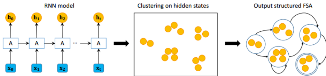
Fig 2.8 Training an RNN model, clustering the RNN’s hidden states and outputting the final structured FSA. [34]
