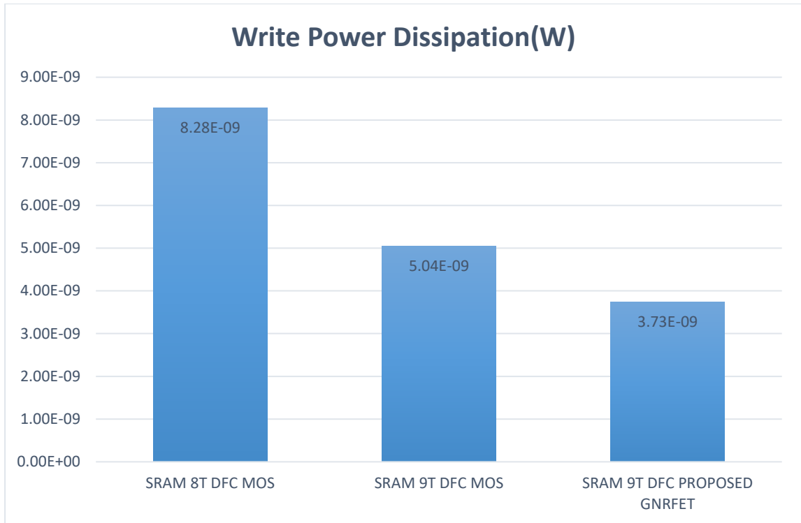
Figure 4.12. Write Mode Power Dissipation for SRAM8T MOS, SRAM9T Power Gated MOS and SRAM 9T Proposed using GNRFET and Power Gating
