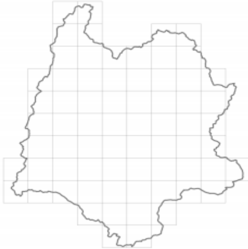
Figure 1.1 Discretization of space in FDM
