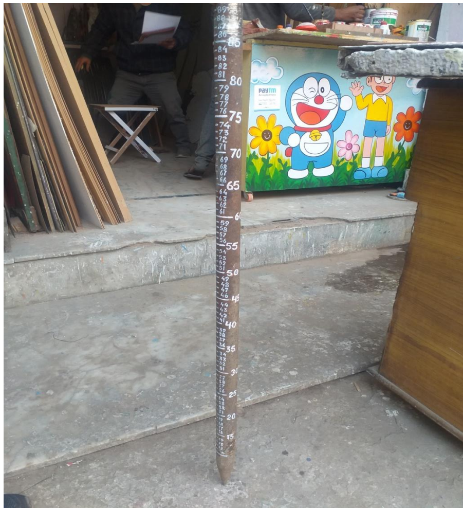
Fig 3.5 Model steel pile
