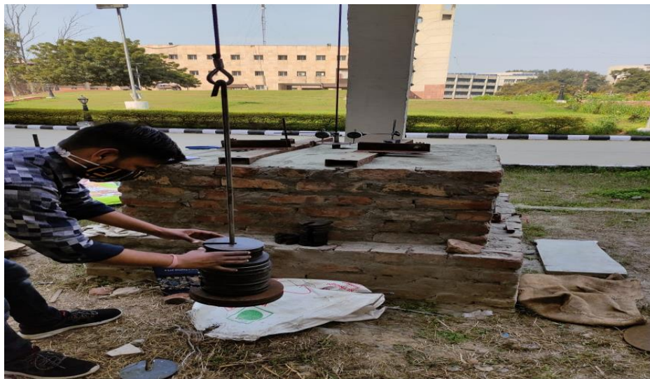
Fig. 4.4 performance of pullout test at \gamma_{(bulk)} = 12.74\text{KN/m}^3
