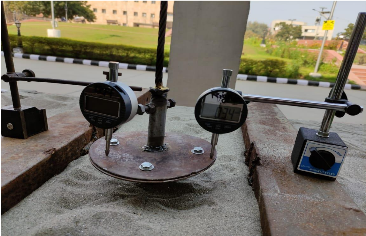
Fig.4.6: Axial pullout readings (in mm) in digital dial gauge
