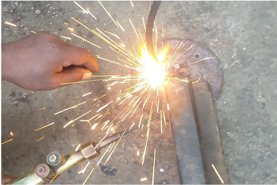
Fig.3.9 Petal welding between wire rope and circular plate
