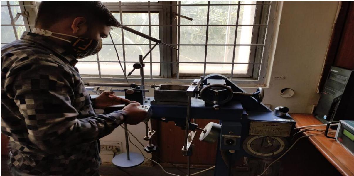
Fig.4.1 Perform D.S.T. in soil mechanics lab
