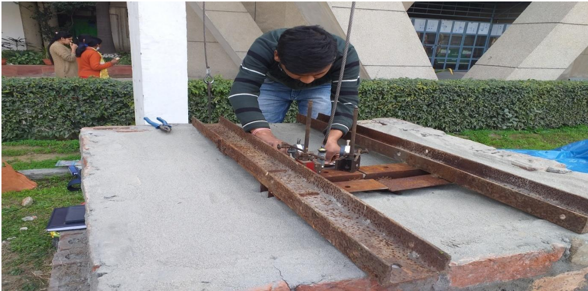
Fig.3.20 set up of two dial gauge stand at equidistant
