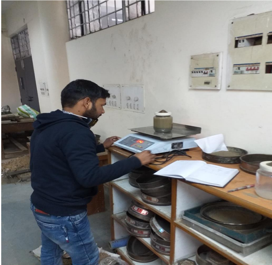
Fig. 4.0 specific gravity of sand by pycnometer method
