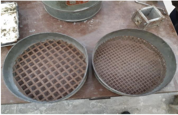
[20mm and 10mm IS sieves respectively]
