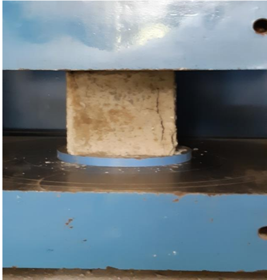
FIG-60 [ cube samples after completion of test with visible cracks] FIG-61
