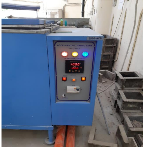
FIG-44 [ the temperature attained 100°C ]
