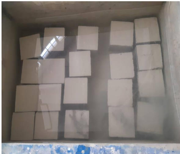
FIG-48 [left 12 cubes in normal curing tank]
