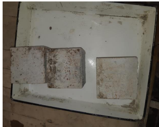
[surface dried samples ready for testing in CTM] FIG-53
