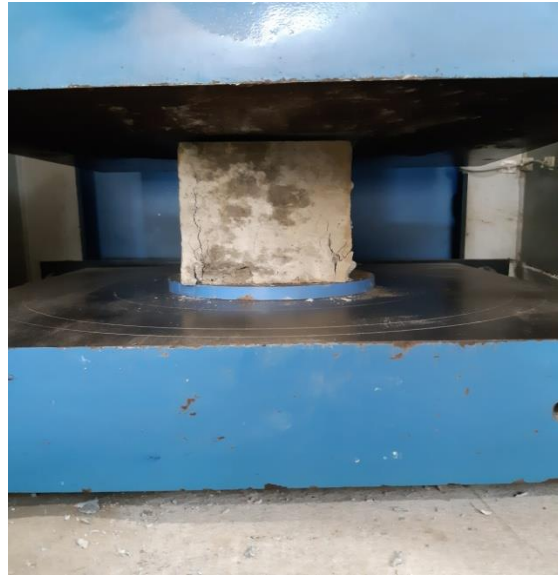
FIG-60 [ cube samples after completion of test with visible cracks] FIG-61
