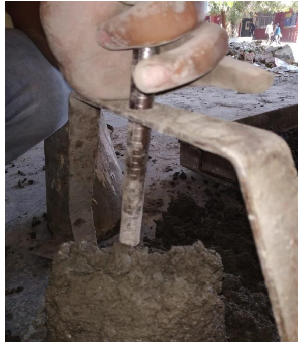
FIG-35 [ Measuring slump ]
