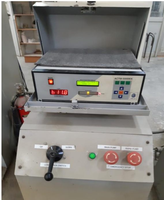
FIG-62 [ during the testing of the cubes reading of load increasing] FIG-63
