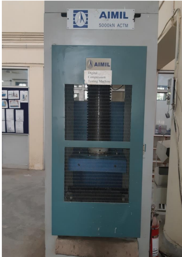
FIG-50 [Compression testing machine]
