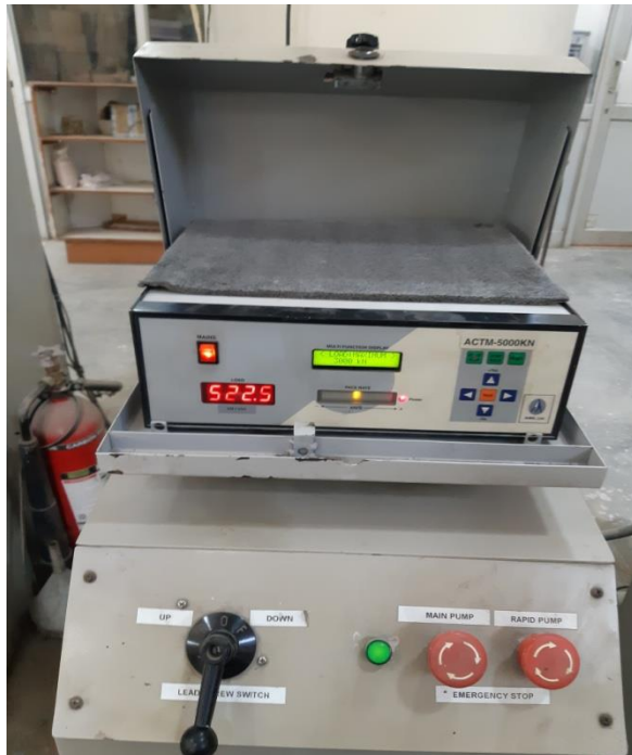
FIG-62 [ during the testing of the cubes reading of load increasing] FIG-63
