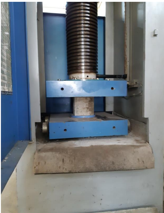
[ cube placed just before the start of test] FIG-59
