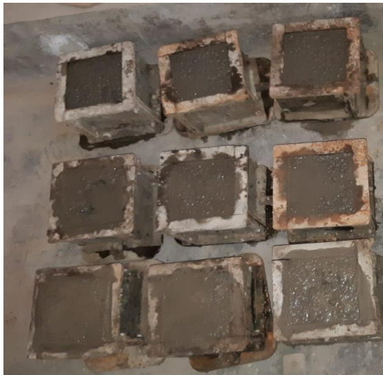
FIG-38 [After complete filling and finishing]
