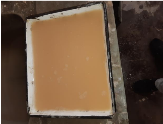
[Fine aggregate left for 24 hrs after step 1 ]
