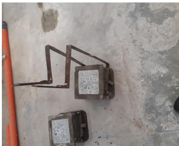
FIG-46 [the mould ready to be lifted]
