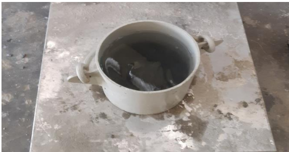
[Aggregates left for 24 hrs soaking]
