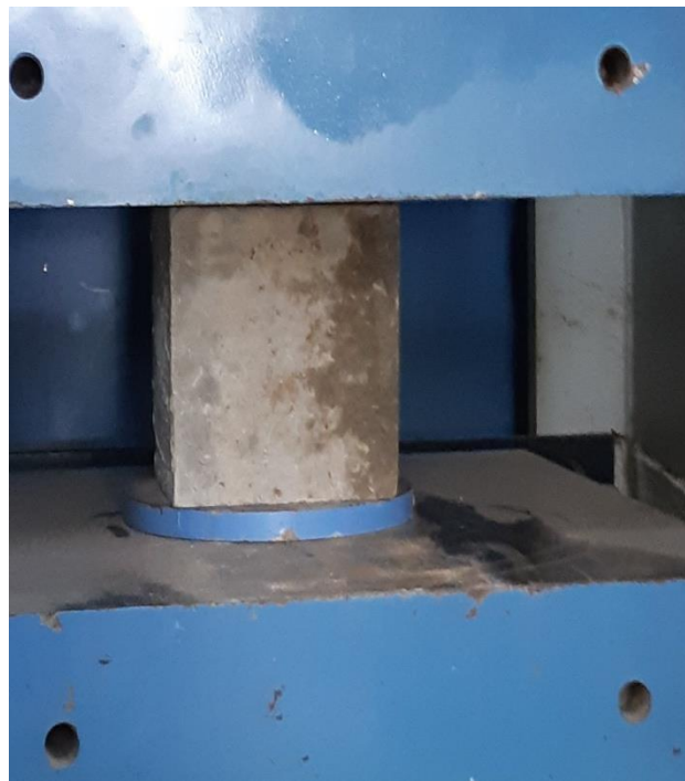
[ cube placed just before the start of test] FIG-59
