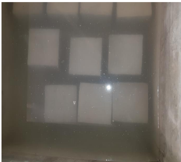
FIG-42 [ N0 MIX cubes in normal curing tank ]
