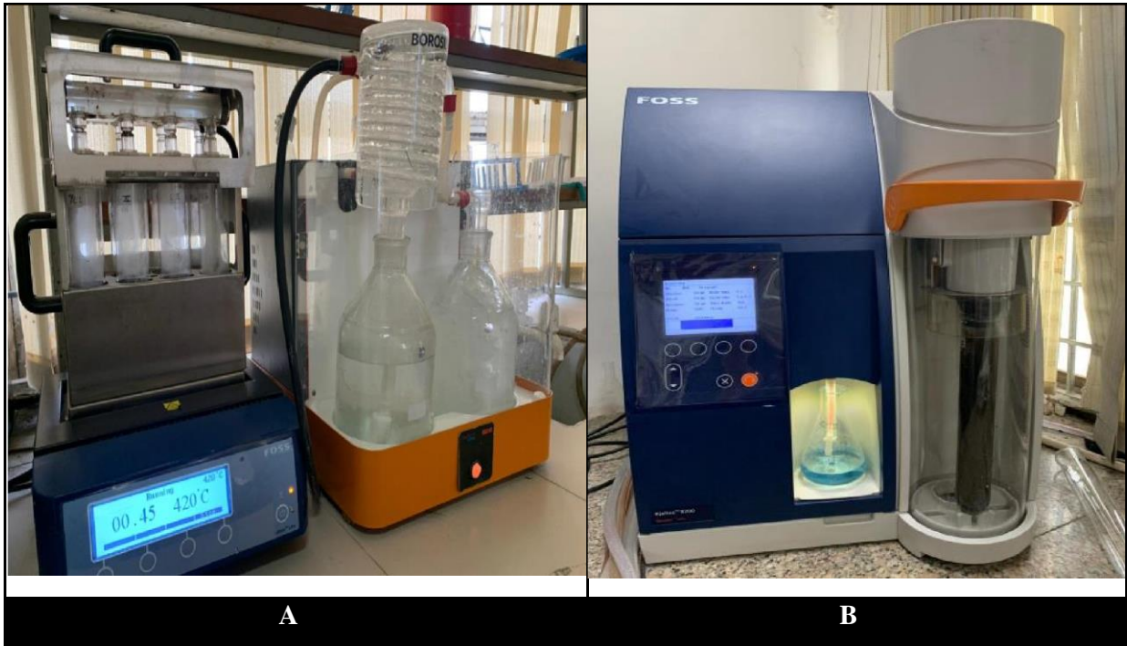
Fig. 2.8 (A) FOSS Kjeldahl block digestion (B) FOSS Kjeltec 8200 steam distillation unit
