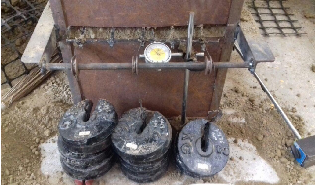
Fig 4.5 : Height of the soil above the geo-grid 8cm and without surcharge
