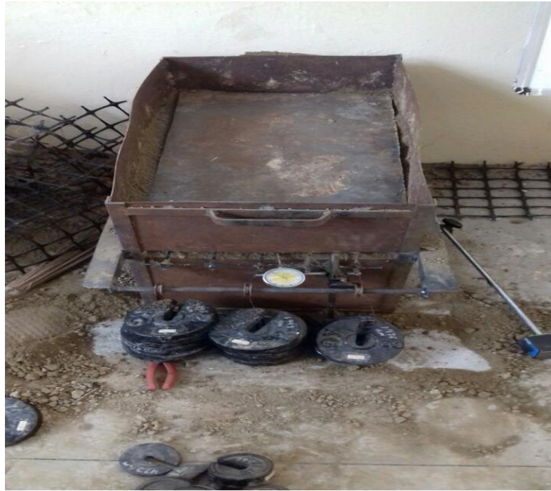
Fig. 4.12 : Top view when surcharge is applied
