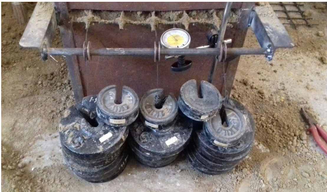
Fig 4.7: Failure when height of the soil above geo-grid 8 cm and surcharge is applied
