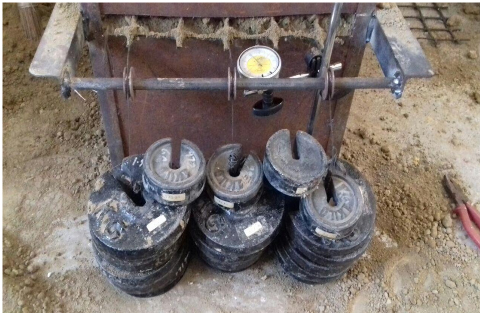
Fig 3.3: Apparatus used to find out the pull -out strength
