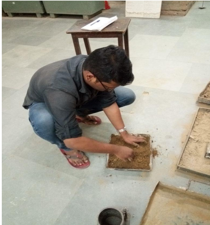
Fig 3.2 (a) Soil sample preparation for proctor test
