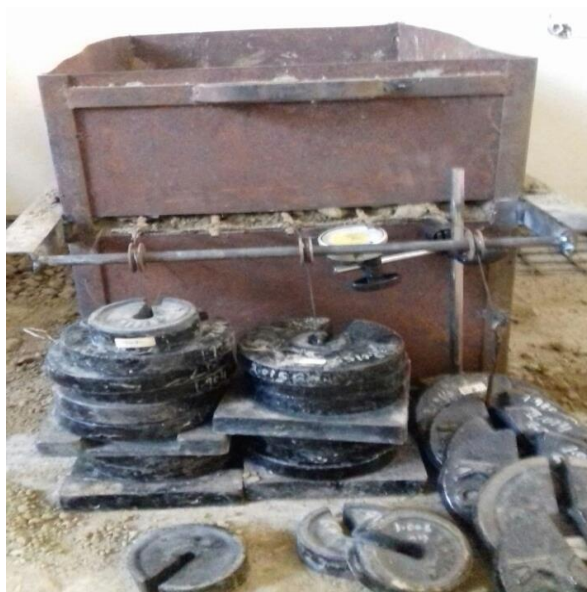
Fig 4.3: surcharge and height of the soil above geo-grid 15 cm over (35 cm x 35 cm)
