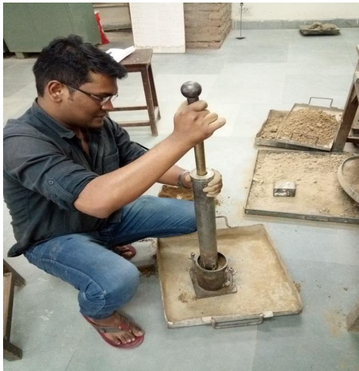
Fig 3.2 (b) Soil sample compaction with the hammer 25 blows for each lawyer of the soil
