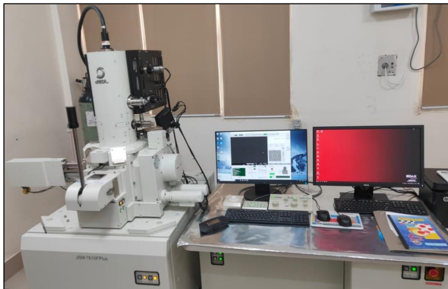
Figure 3.3 JEOL JSM-7610F Plus for FESEM
