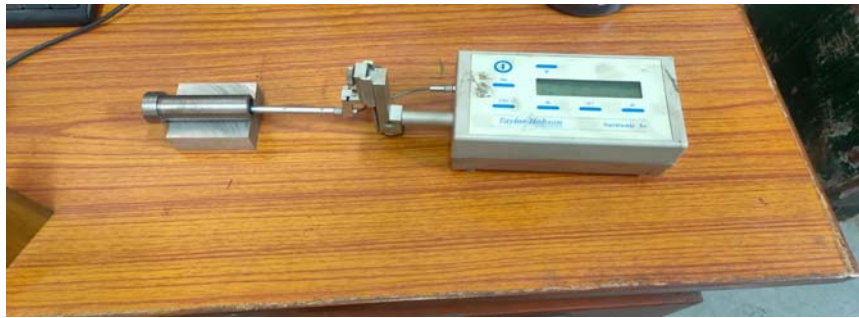
Fig. 6.50 Surface roughness measurement of Internal Spline by TalySurf
