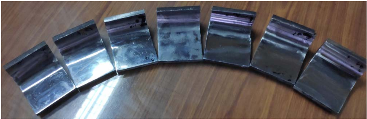
Fig. 7.11. Steel Specimen Finished with Viscoelastic Magnetic Abrasive Medium
