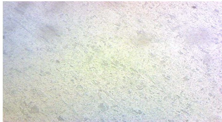
Fig.7.16 Etched Aluminium piece finished with VEMAF Process 500X
