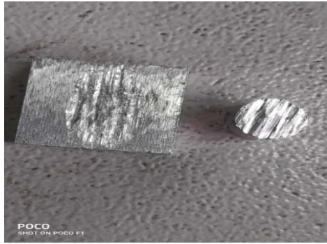
Fig.8.17. Aluminum Rough Specimen after wear
