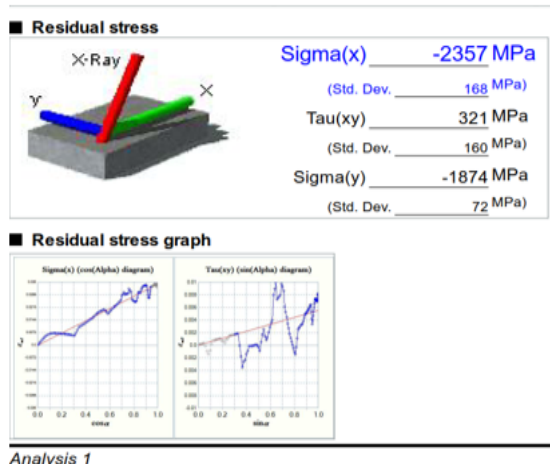
Graph.7.36 Residual stresses of Brass specimen 5 Before and After finishing
