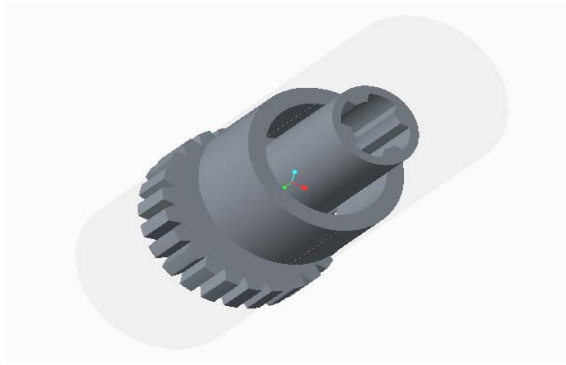
Fig.6.38 Solid model of Spline shaft and the Arc magnet
