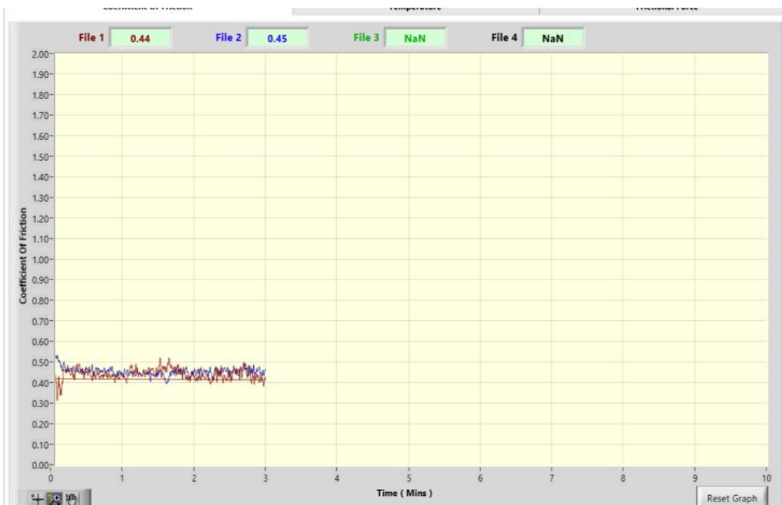
Graph.8. 32. Comparison of Coefficient of friction of Steel Rough and finished specimen L7
