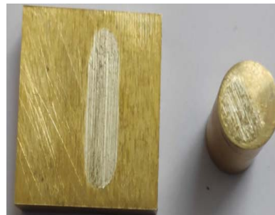
Fig. 8.13 Brass Rough Specimen after wear Fig. 8.14 Brass Finished specimen after Wear
