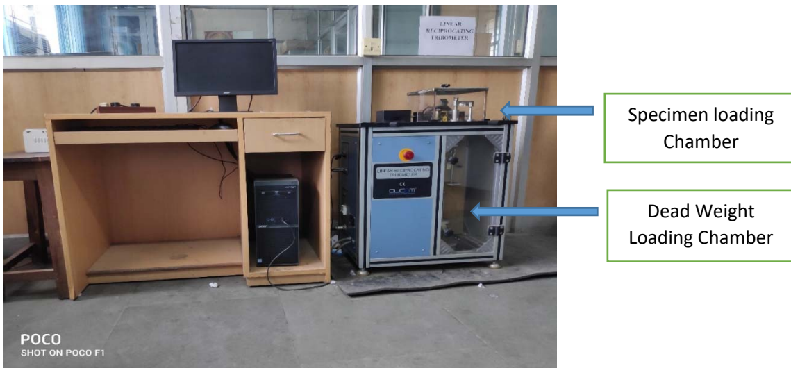
Fig. 8.6 Linear Reciprocating Tribometer
