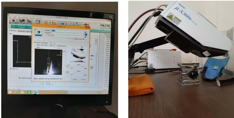
Fig.7.7. Residual Stress analyzer and Monitor
