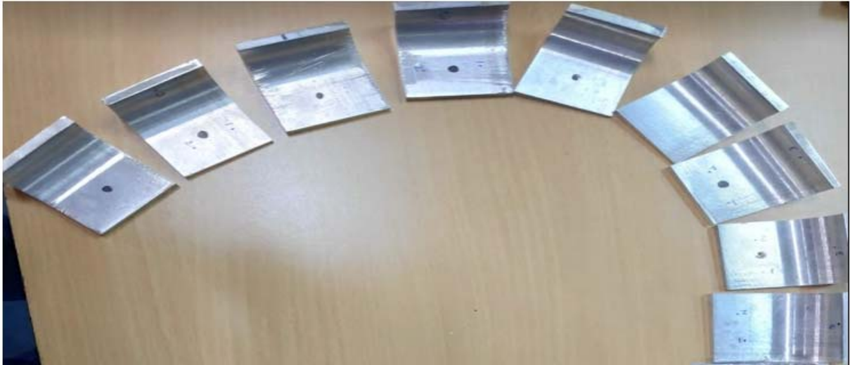
Fig.7.15. Aluminum Specimen finished with Viscoelastic Magnetic Abrasive Medium
