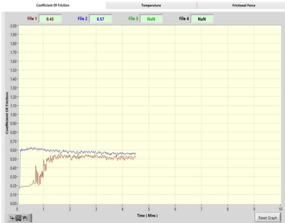
Graph.8.33 Comparison of Coefficient of friction of Steel Rough and finished specimen L8
