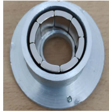
Fig 6.23 Bottom Cover plate Fig. 6.24 Top Cover plate Fig.6.25 Magnet Assembly
