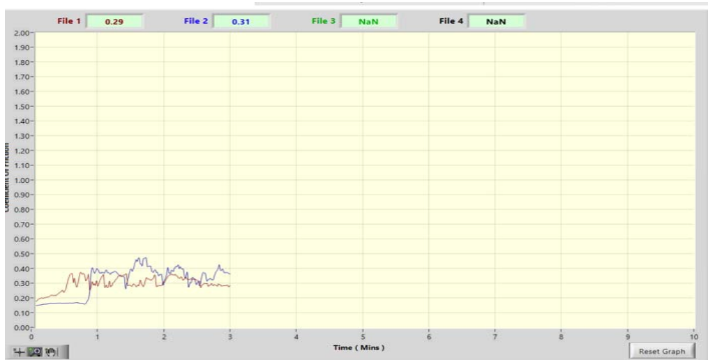
Graph.8.9. Comparison of Coefficient of friction of Brass Rough and finished specimen L1
