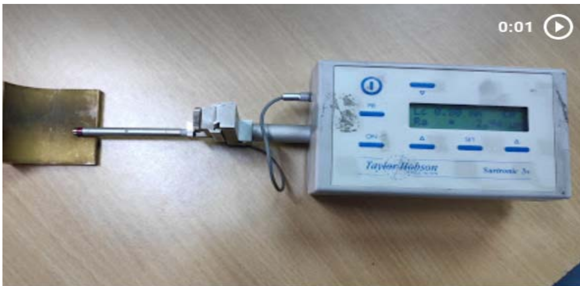
Fig.7. 10. Surface roughness Measurement of Unfinished Brass Specimen
