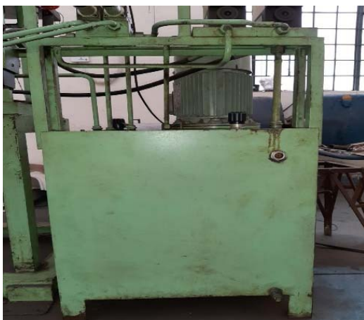
Fig.6.3 Hydraulic Power Pack
