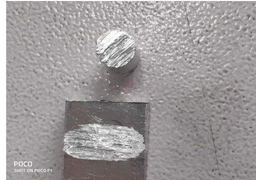
Fig.8.18. Aluminum finished Specimen after wear
