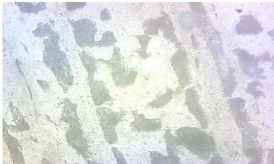
Fig. 7.12. Etched Steel Specimen finished with VEMAF Process 500X
