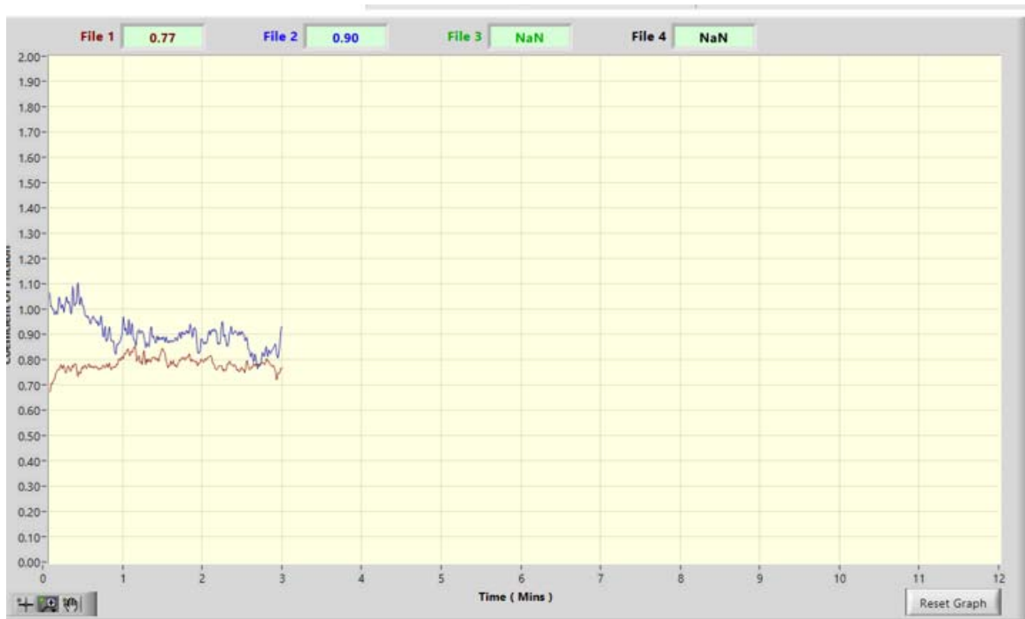
Graph.8.43. Comparison of Coefficient of friction of Steel Rough and finished specimen L1
