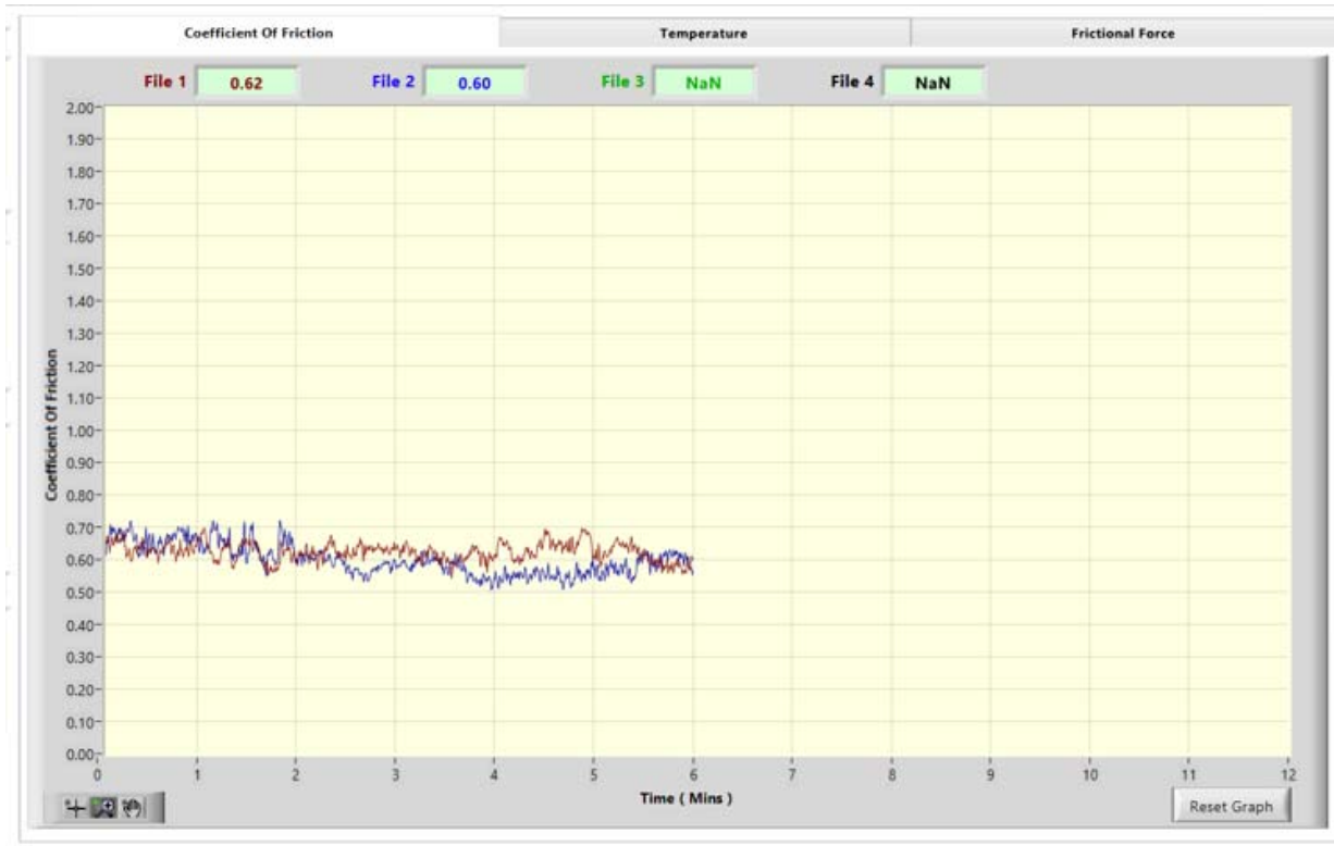
Graph.8.46. Comparison of Coefficient of friction of Steel Rough and finished specimen L4
