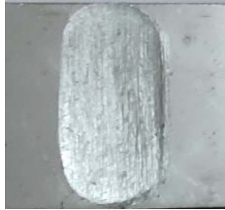
Fig. 8.15. M S Rough Specimen after wear Fig. 8.16 M S Finished Specimen after wear
