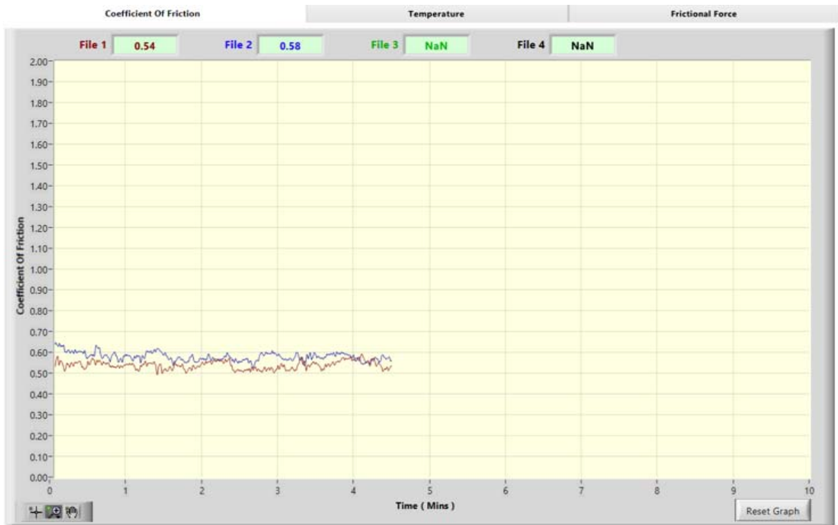
Graph.8.50. Comparison of Coefficient of friction of Steel Rough and finished specimen L8
