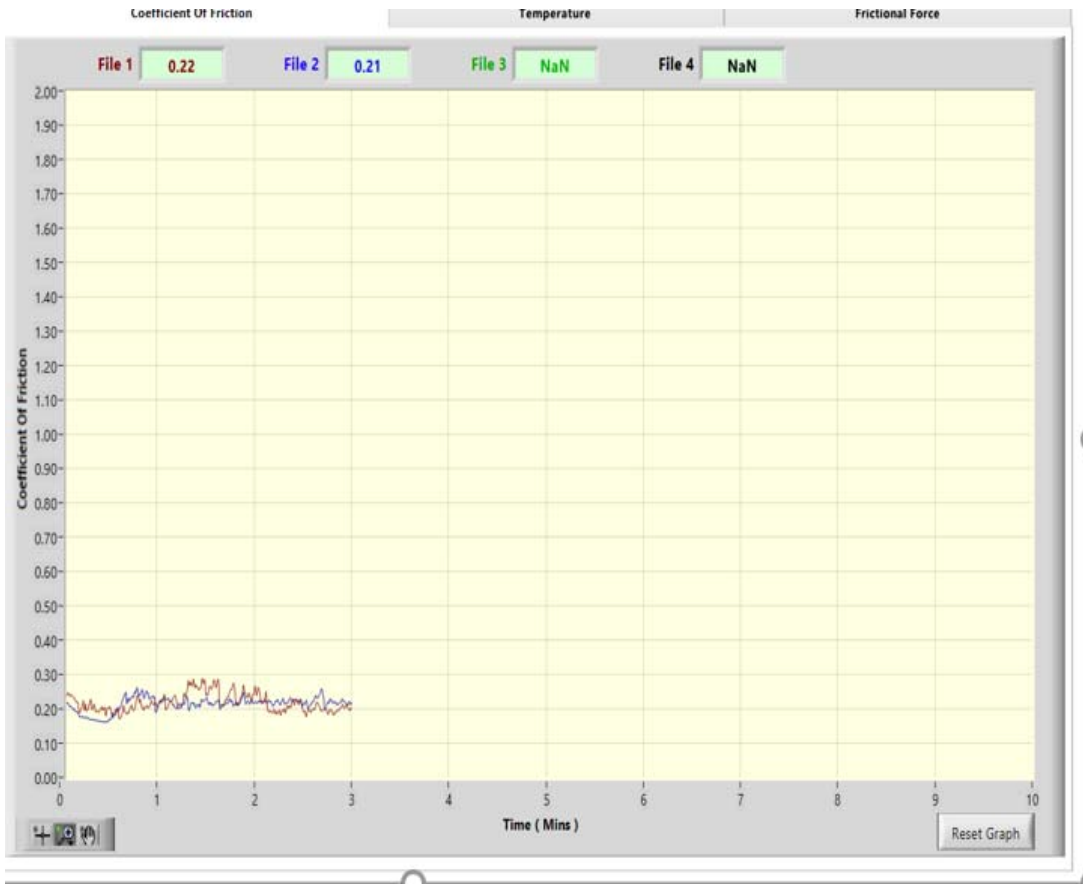
Graph.8.15. Comparison of Coefficient of friction of Brass Rough and finished specimen L7
