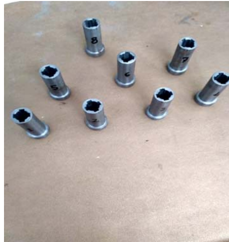
Fig.6.52.Finished Internal Spline Shafts
