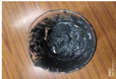
Fig. 3.11. Silicone Oil-based Viscoelastic Magnetic Abrasive Medium
