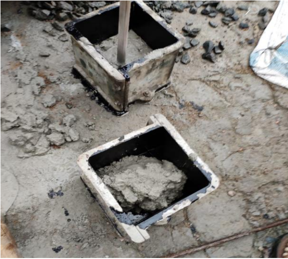
Figure 4.1 Filling of concrete in cube
