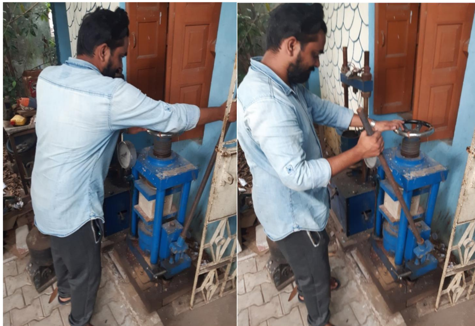
Figure 10: Testing Of Cubes On CTM
