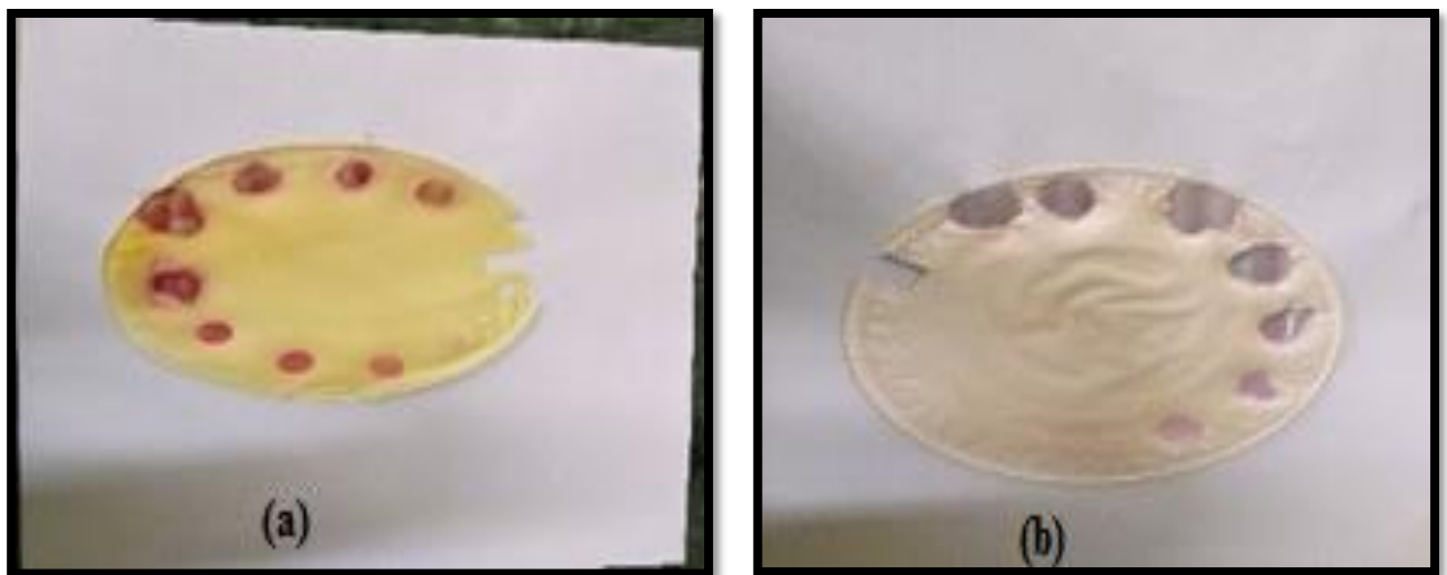
Figure 4.3: Color Parameters of (a) EC- MO Film (b) EC- MR Film, with Varying Percentage of Acid
