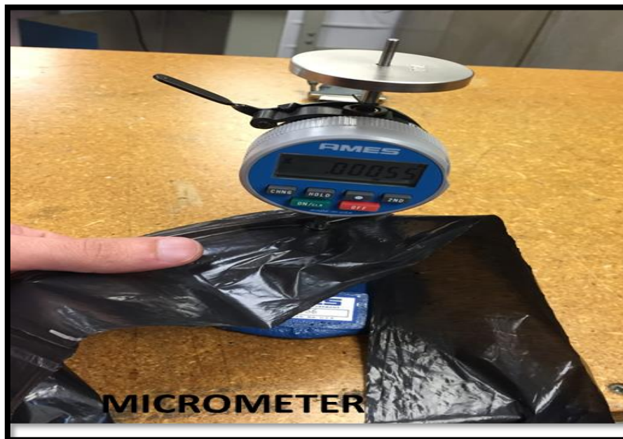
Figure 2.5: Micrometer Measurement of th Thickness of the Plastic Film
