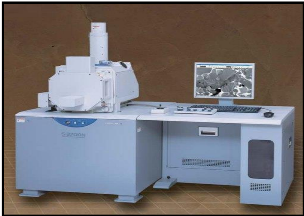
Figure 2.4: Scanning Electron Microscope (Hitachi S-3700N, Japan)
