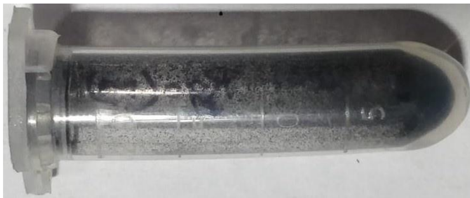
Fig 3.2. Image showing rGO@ZnO nanocomposite
