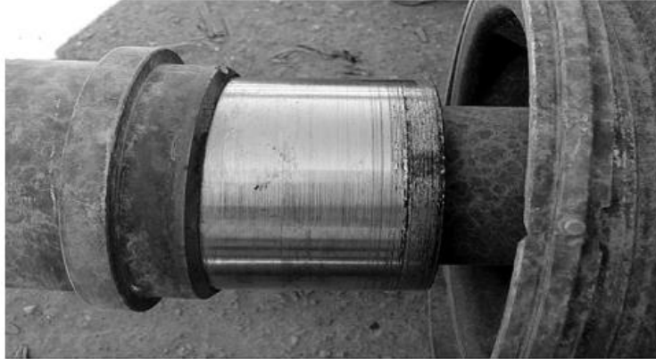
Fig.1.5 Worn shafts of gas turbine [12]
