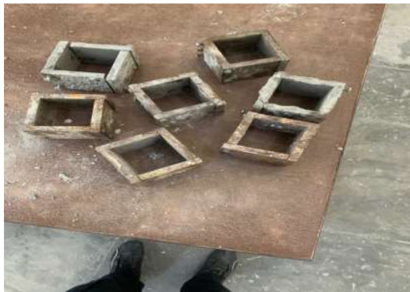
Fig 3.4 - Cubicle moulds before and after tightening
