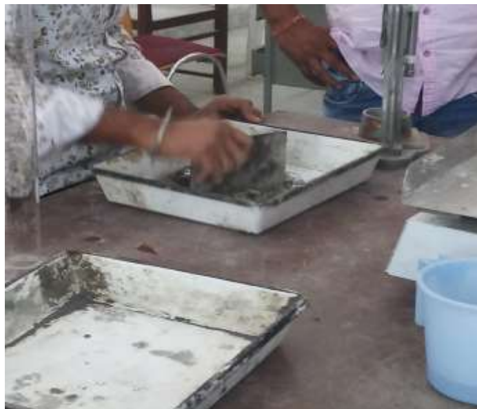
Fig 3.6 - Mixing of cement, sand and water manually
