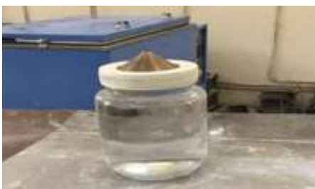
[pycnometer filled with water only]
