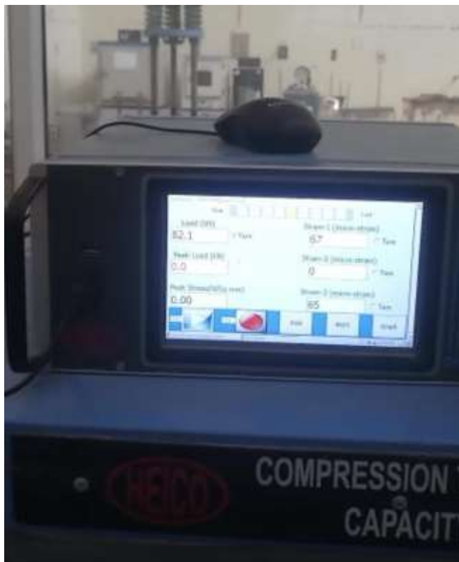
Fig 3.12 - Monitor showing applied load
