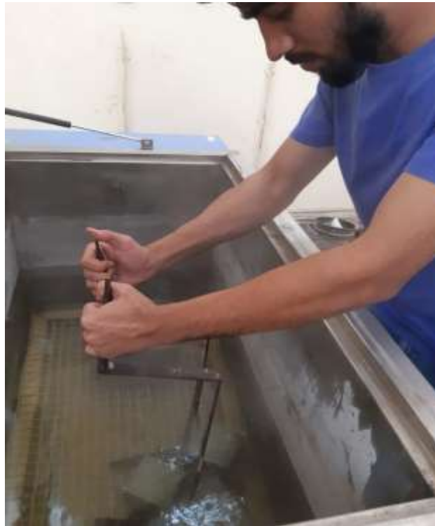
Fig 3.9 - Placing of mortar cubes in the tank
