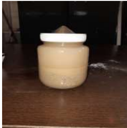
[Fine aggregate left for 24 hrs after step 1]
