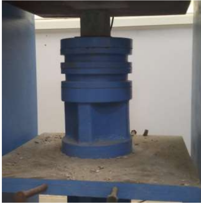
Fig 3.11 - Placing of mortar cube in CTM
