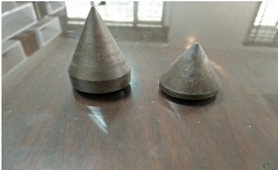
Figure 5: Cones of a static cone penetration test
