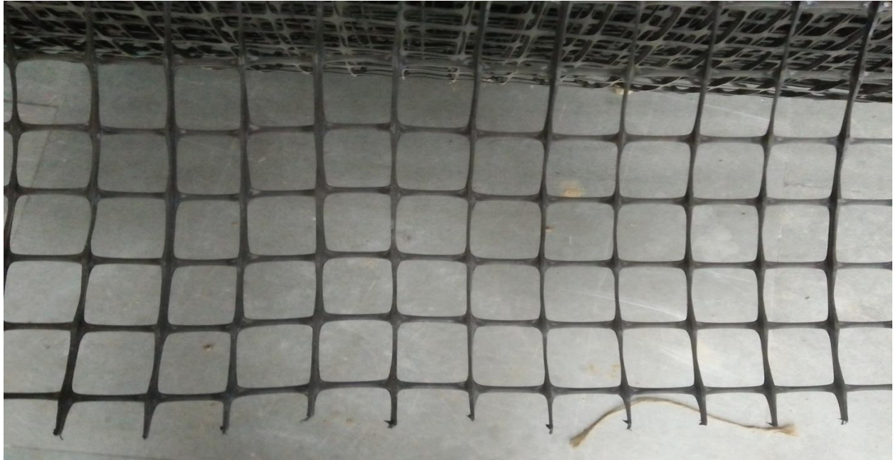
Figure 1: Biaxial square geogrid
