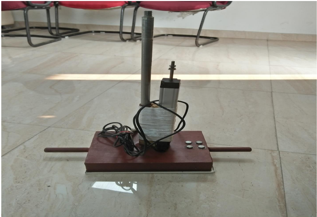
Figure 3: Static cone penetrometer
