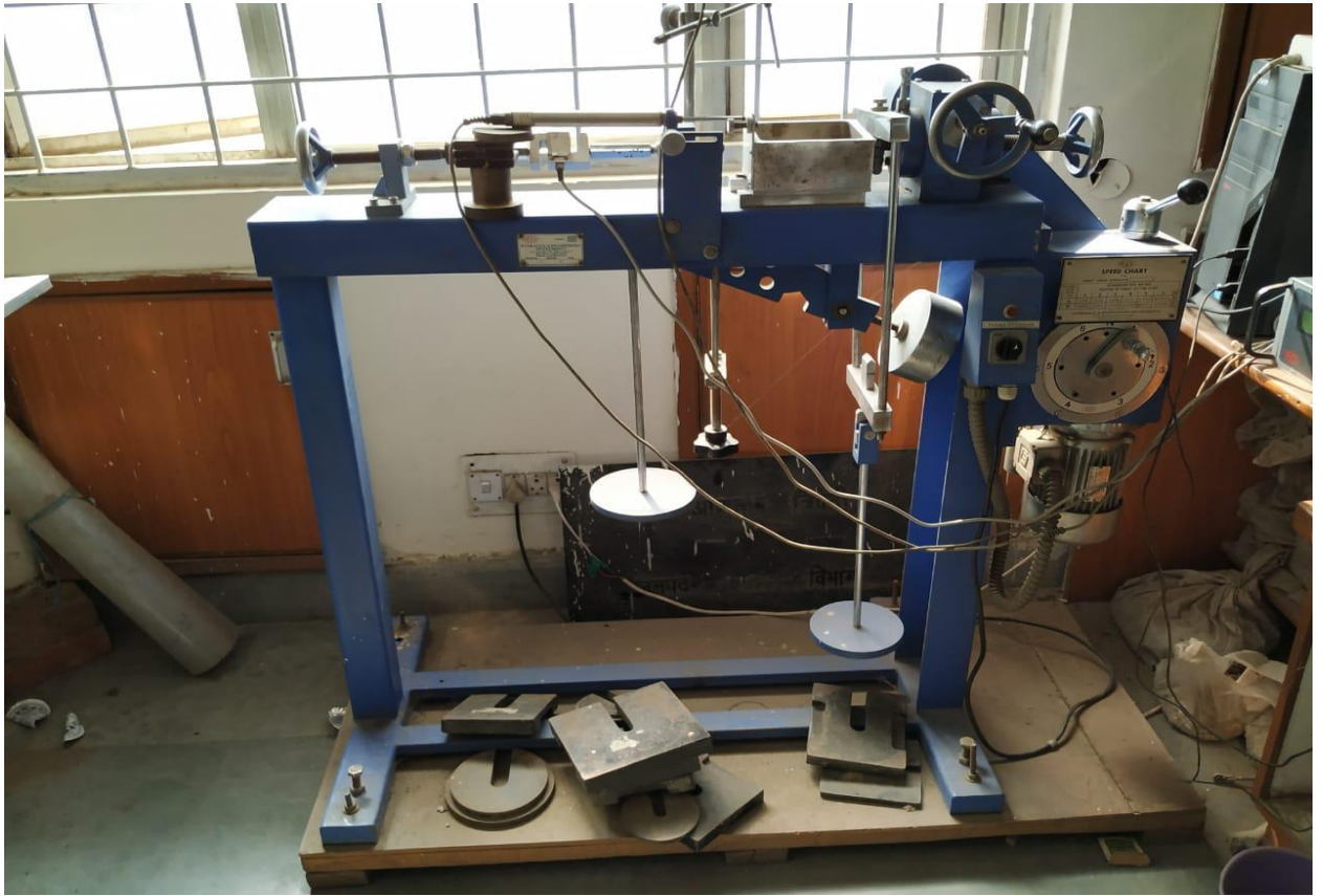
Figure 9: Direct shear test apparatus
